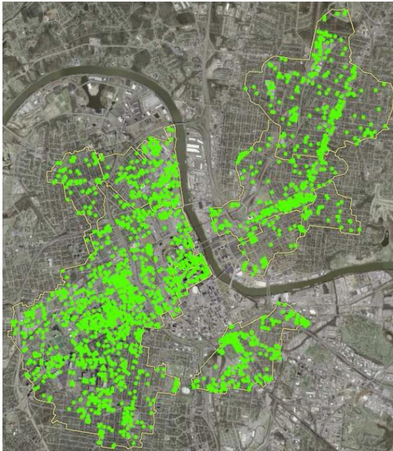
Figure 3: Potential green roof locations in the Nashville/Davidson Co. combined sewer system district<sup>45</sup>.
