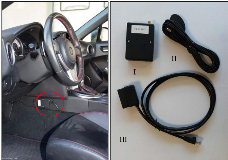
Figure 4.2 (Left) i2D device connected to the vehicle. (Right) I. the device II. antenna III. OBD-II connector cable
