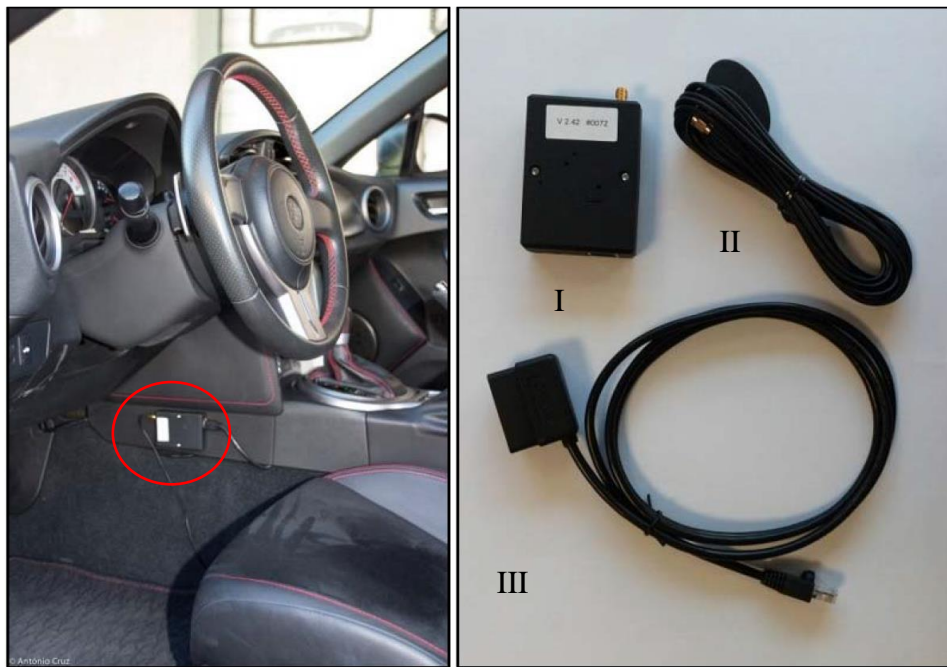
Figure 5.1. (Left) i2D device connected to the vehicle. (Right) I. the device II. antenna III. OBD-II connector cable
