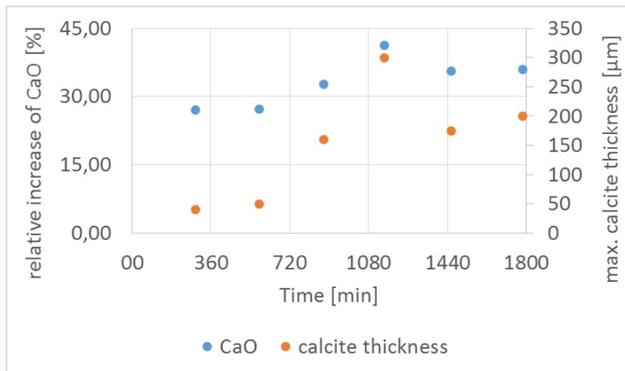
Figure 8: Relative increase of the CaO concentration of the crack surfaces (left) and maximum thickness of the calcite layer (right) related to the time the specimens were flown by steam.
