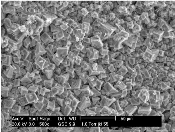
Figure 6: ESEM picture of a CEM III (w/c 0.3) specimen (55) flown by steam.
