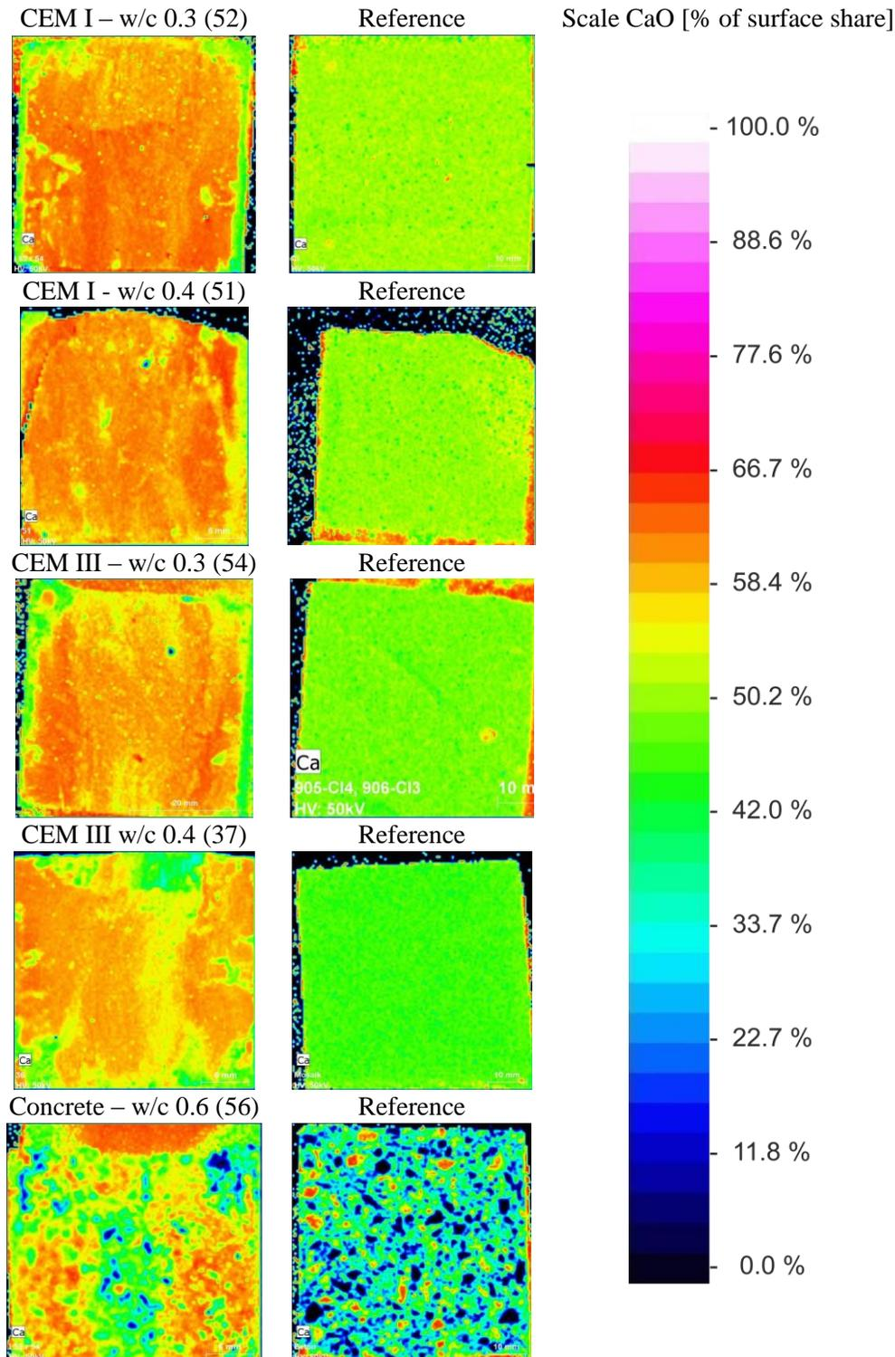
Figure 5:  $\mu$ -RFA surface scans showing one example from each steam flow material and the related reference. Flow direction from top to bottom.
