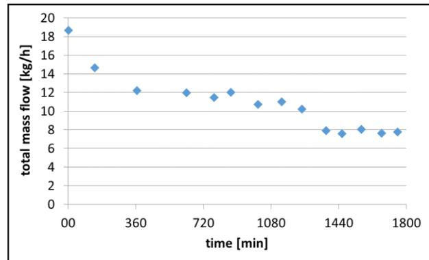
Figure 3: Measured flow amount and their associated crack width. Crack length = 4 cm, experiment time of a long term test run wideness = 3 cm.
