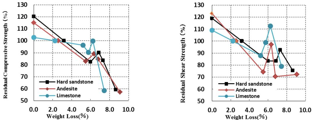
Figure 3 Relationship between weight loss and residual ratio of compressive/shear strength (case A)
