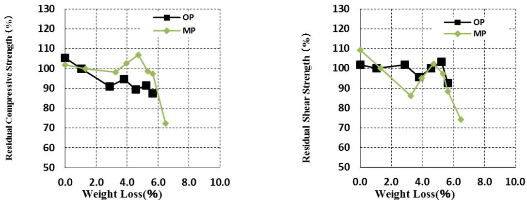
Figure 4 Relationship between weight loss and residual ratio of compressive/shear strength (case B)
