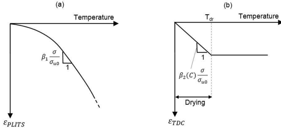
Figure 4 Temperature development of the two components of LITS: the moisture independent PLITS  $\varepsilon_{plits}$  and the moisture dependent strain TDC  $\varepsilon_{tdc}$
