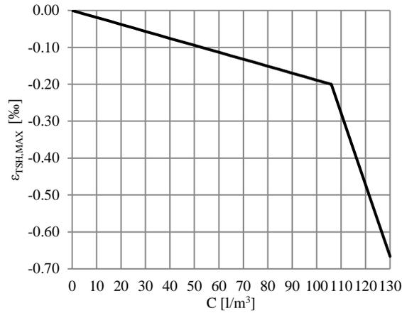
Figure 6 Maximum expected transient shrinkage  $\varepsilon_{tsh,max}$  as a function of the initial water content.
