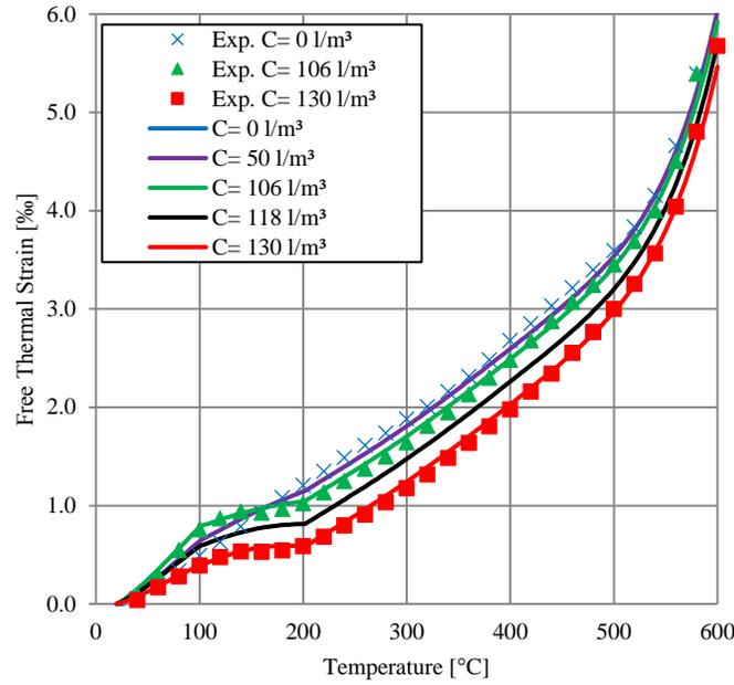
Figure 9 Experimental FTS curves and numerical results
