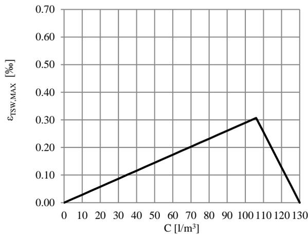
Figure 7 Maximum expected transient swelling  $\varepsilon_{tsw,max}$  as a function of the initial water content.
