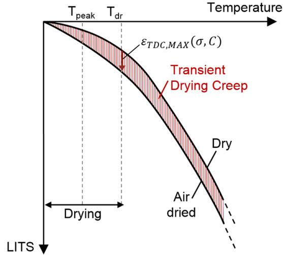
Figure 2 LITS developing in dry and air dried concrete. Schematic representation of the transient drying creep contraction (in red) occurring for air dried concrete.
