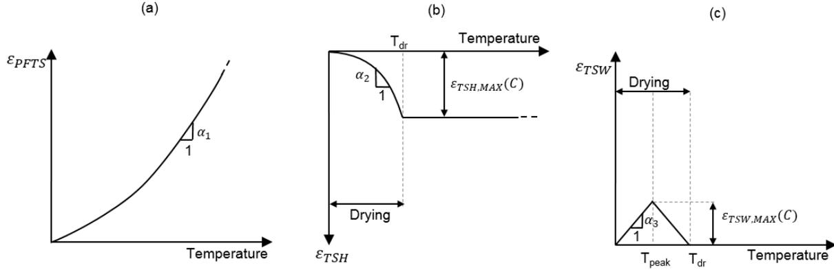
Figure 3 Temperature development of the three components of FTS: the moisture independent PFTS  $\epsilon_{pfts}$  and the moisture dependent strain components TSH  $\epsilon_{tsh}$  and TSW  $\epsilon_{tsw}$
