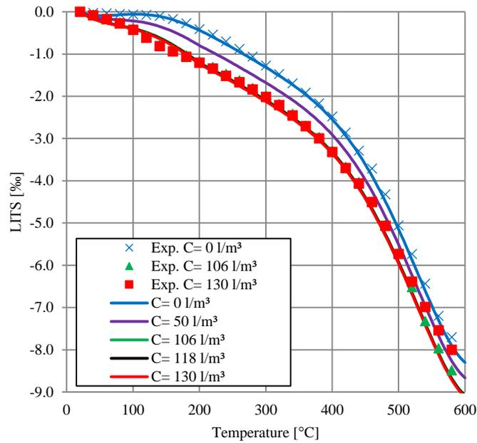
Figure 10 Experimental LITS curves and numerical results
