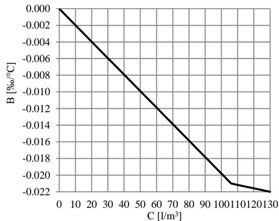
Figure 8 TDC coefficient  $B$  as a function of the initial water content.
