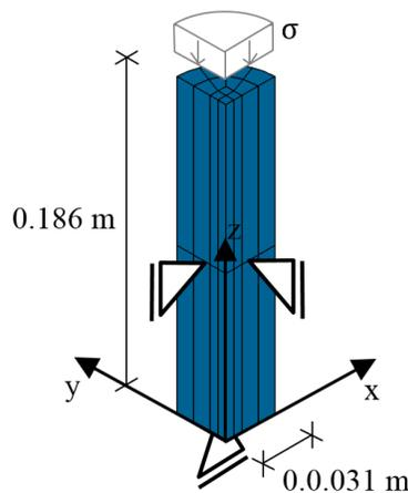
Figure 5 Mesh, boundary and loading conditions defined for modelling the uniaxial transient tests reported in (Khoury et al., 1985a)
