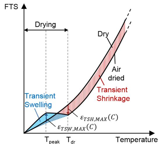
Figure 1 FTS developing in dry and air dried concrete. Schematic representation of the transient shrinkage contraction (in red) and transient swelling effect (in blue) occurring for air dried concrete.
