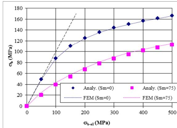
Fig. 5: Validation of the FEM protocol through comparison to an analytical solution
