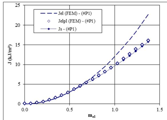
**Fig. 8:** J calculation for the secondary bending moment without pressure
