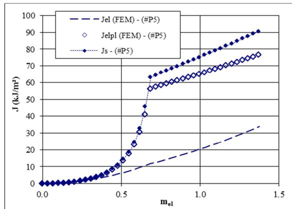
**Fig. 10:** J calculation for 50% primary bending moment cumulated with pressure (non-radial configurations)
