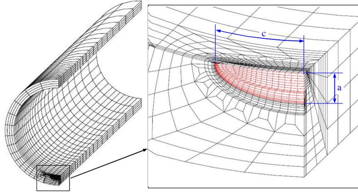
**Fig. 6:** Mesh of the cracked pipe with an internal semi-elliptical surface defect (CDSI)
