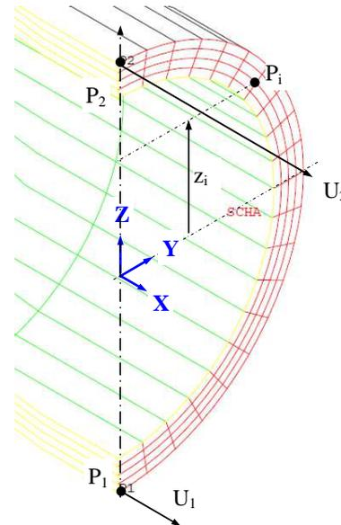
Fig. 4: Kinematic relation in the loaded section
