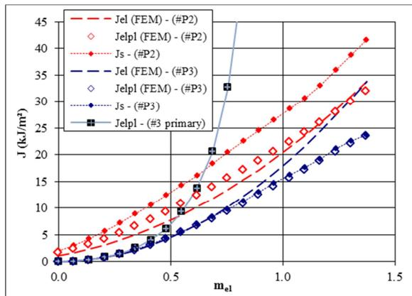
**Fig. 9:** J calculation for the secondary bending moment cumulated with pressure (radial and non-radial configurations)
