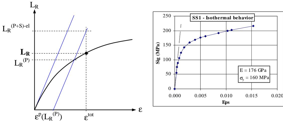
**Fig 2:** On left: Representation of the scheme in a stress-total strain diagram
