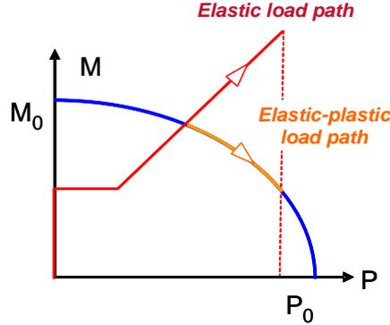
*Fig. 1: Illustration of the secondary bending moment relaxation*
