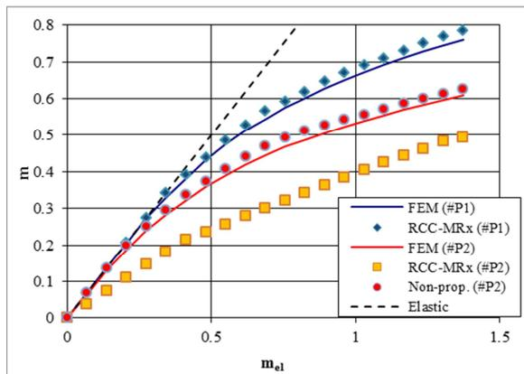
**Fig. 7:** Elastic-plastic bending moment calculation
