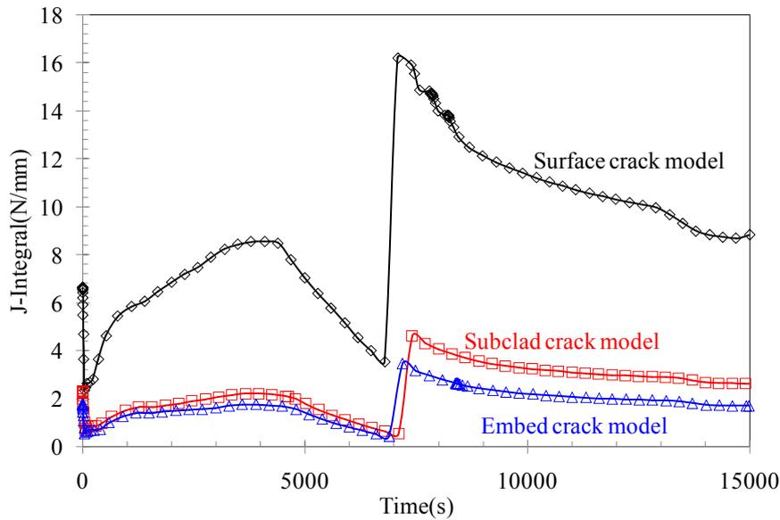
Figure 5 The maximum J-integral for different crack models
