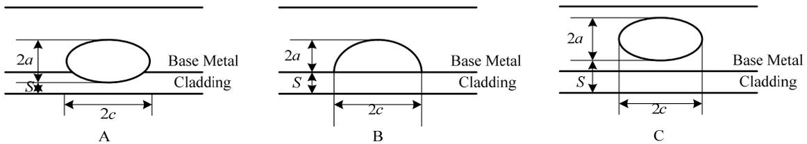
Figure 2 The subsurface crack in clad components
