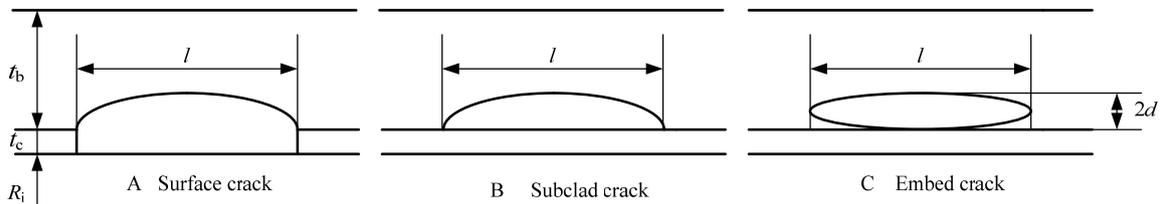
Figure 3 crack size and characterization in clad component
