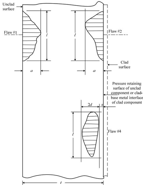
Figure 1 Planar flaws near the interface in clad components
