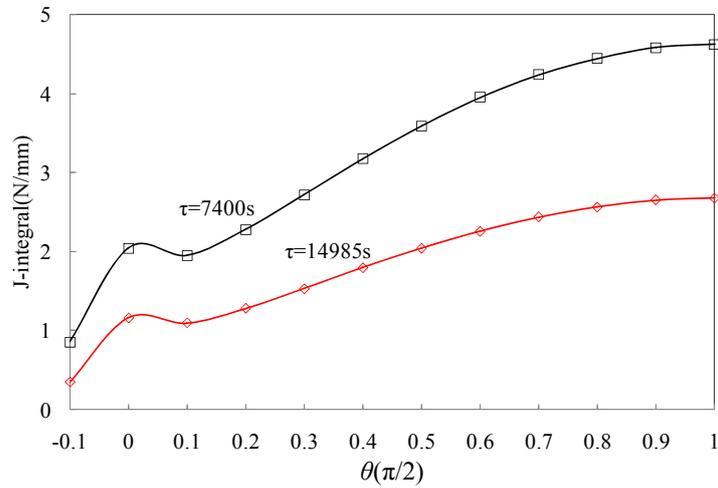
b) Surclad semi-elliptical crack
