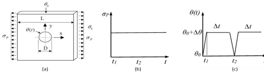
Figure 1. (a) Geometry of the 3D plate and loading condition, (b) uniaxial tensile load, and (c) cyclic thermal load.
