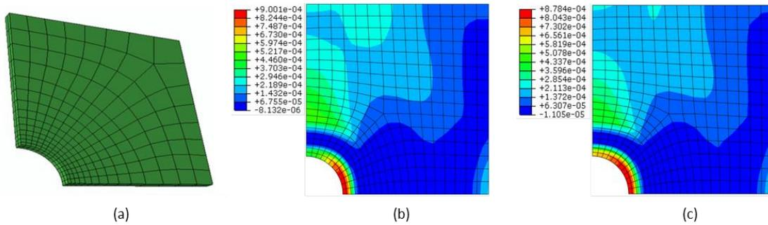
Figure 3. (a) Meshed FE model and FE model verification; (b) equivalent creep strain for 10hrs dwell time from the LMM and (c) equivalent creep strain for 10hrs dwell time from the SBS analysis.
