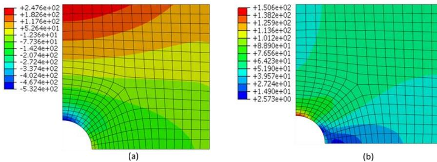
Figure 6. Linear elastic stress solutions: (a) stress component,  $\sigma_{11}$ , from thermal stress only with  $\Delta\theta=0.7$  and (b) stress component,  $\sigma_{11}$ , from mechanical stress only with  $\sigma_p=0.5\sigma_{p0}$ .
