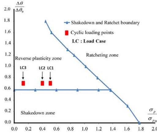
Figure 2. Shakedown and ratchet limit curve for the holed plate with the cyclic thermal load and the constant mechanical load without the creep effects.
