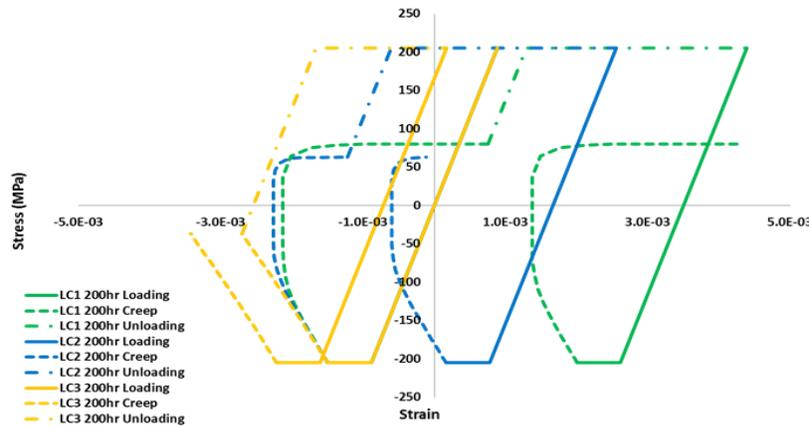
Figure 8. Response of steady state stress-strain loop corresponding to load cases 1, 2, and 3 for dwell time 200hrs
