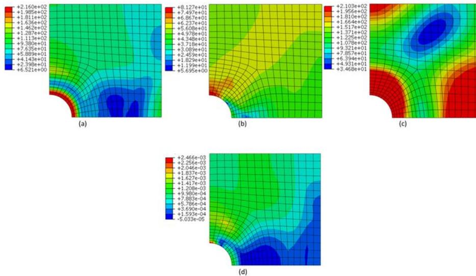
Figure 4. Equivalent von-Mises stress distribution per loading instance with load case 1 for dwell time 200hrs at the last load cycle; (a) loading, (b) creep, (c) unloading, and (d) equivalent creep strain increment at dwell
