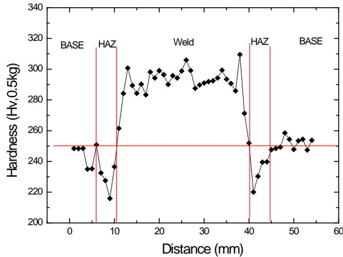
Figure 2. Vickers micro-hardness for BM, WM, and HAZ of Gr. 91 steel.
