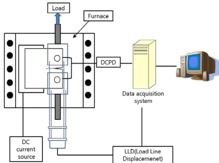
Figure 1. A schematic diagram for the CCG tests.
