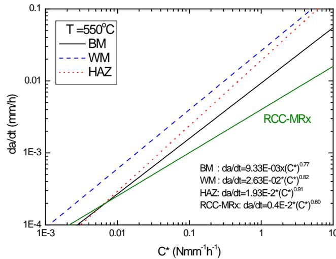
Figure 5. Comparison of CCGR curves for the BM, WM, and HAZ
