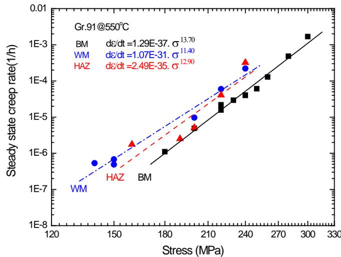
Figure 3. Comparison of the steady state creep rate for the BM, WM, and HAZ at 550°C.
