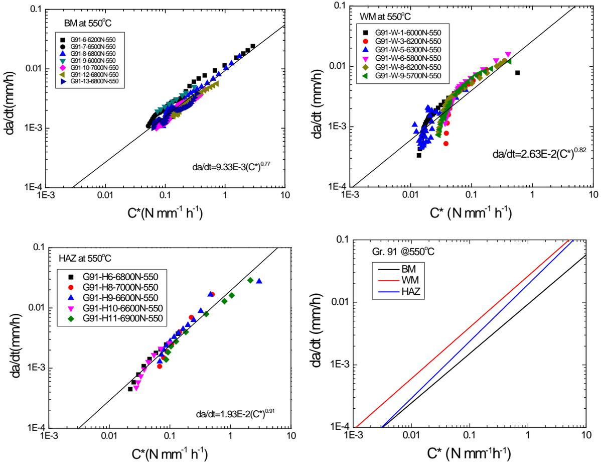
Figure 4. Plot of  $C^*$  vs. CCGR for the BM, WM, and HAZ
