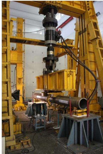
Figure 3: A view of fracture test set-up for a DMW pipe weld
