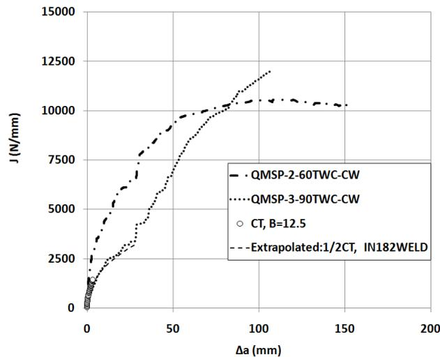
Figure 6. J-R curves of cracked pipe weld (through wall crack in centre of weld) and compact tension specimen.
