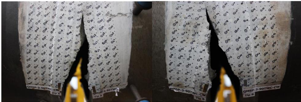
Figure 5. Close-up views of crack location after the fracture for QMSP-3-90TWC-CW
