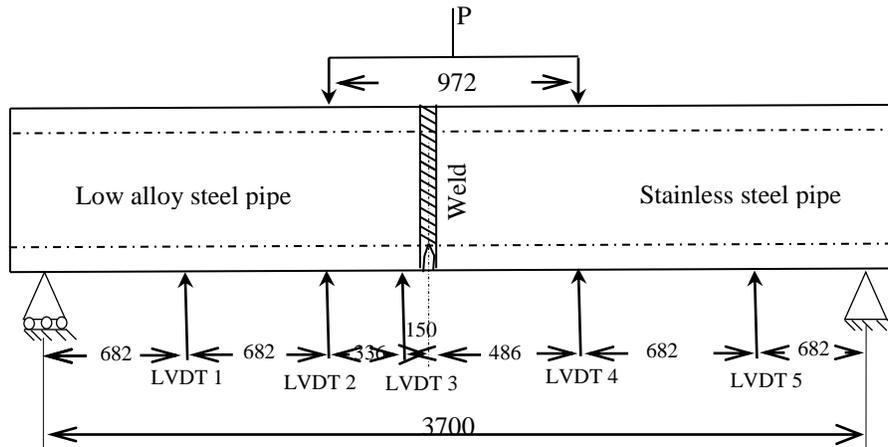
Figure 2. Details loading scheme and LVDT locations for deflection measurements during the fracture test on the specimen. **Note:** All dimensions are in mm
