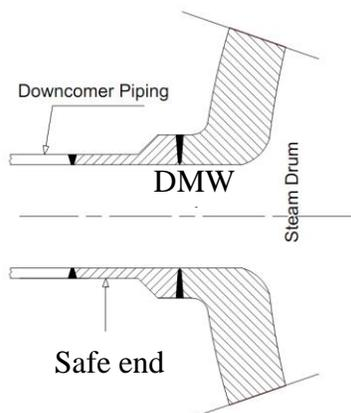
Figure 1. Schematic of steam drum nozzle welded to downcomer piping
