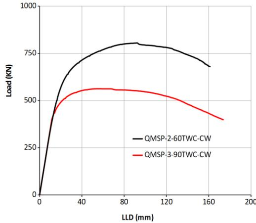
Figure 4. Load vs. LLD for pipe with through-wall crack in centre of weld
