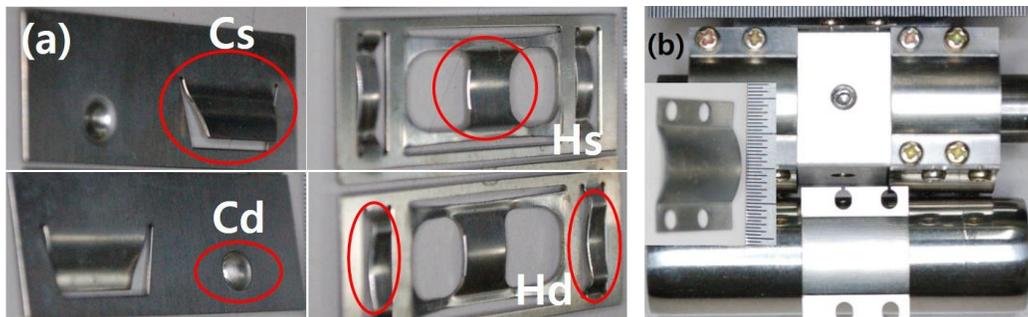
Figure 1. (a) Spacer grid candidates for dual-cooled annular fuel and (b) simulated outer fuel rod specimen used in this study.
