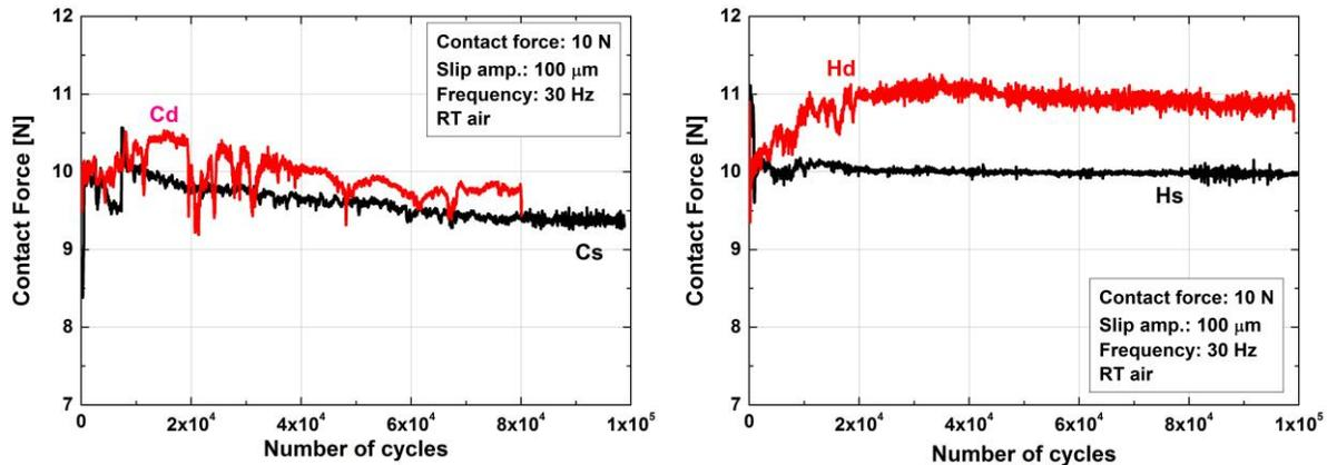
Figure 5. Variation of initial contact force with increasing number of fretting cycles.
