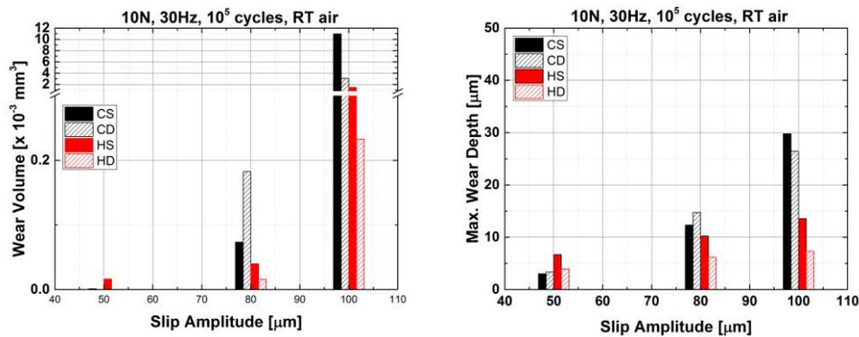
Figure 3. Variation of wear volume and maximum wear depth with increasing slip amplitude.
