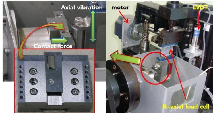
Figure 2. Schematic view of fretting wear tester for examining wear resistance of spacer grid.
