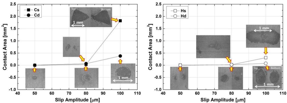
Figure 4. Worn surface morphology and calculated worn area after the fretting wear tests.
