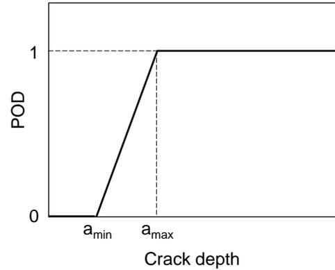
Figure 2 POD curve expressed by linear interpolation between  $a_{min}$  and  $a_{max}$
