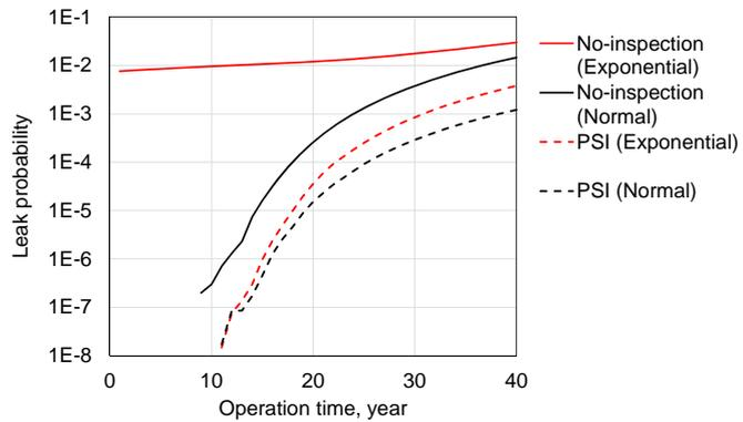
Figure 7 Effect of difference in distribution of initial crack depth on leak probability (600A pipe)
