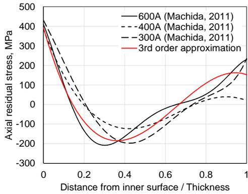
Figure 6 Weld residual stress distribution
