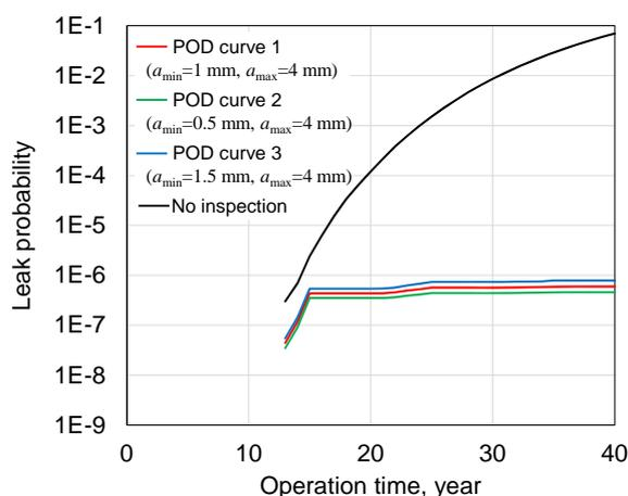
Figure 9 Effect of difference in  $a_{min}$  used in POD curve on leak probability
