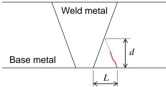
Figure 5 Distance between weld fusion line and crack
