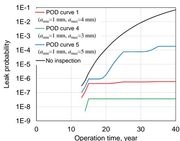
Figure 10 Effect of difference in  $a_{max}$  used in POD curve on leak probability
