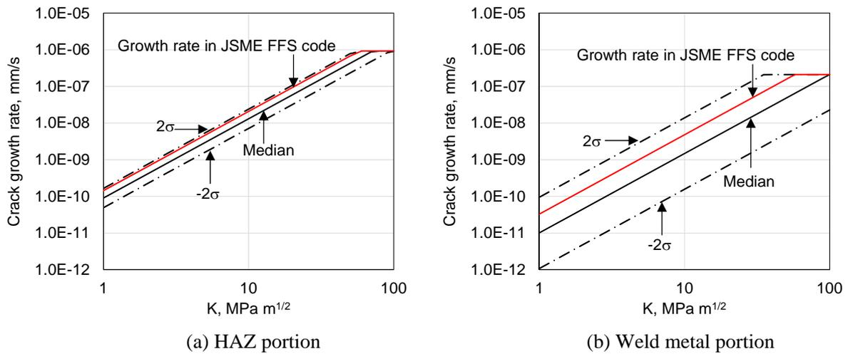
Figure 4 SCC crack growth rates
