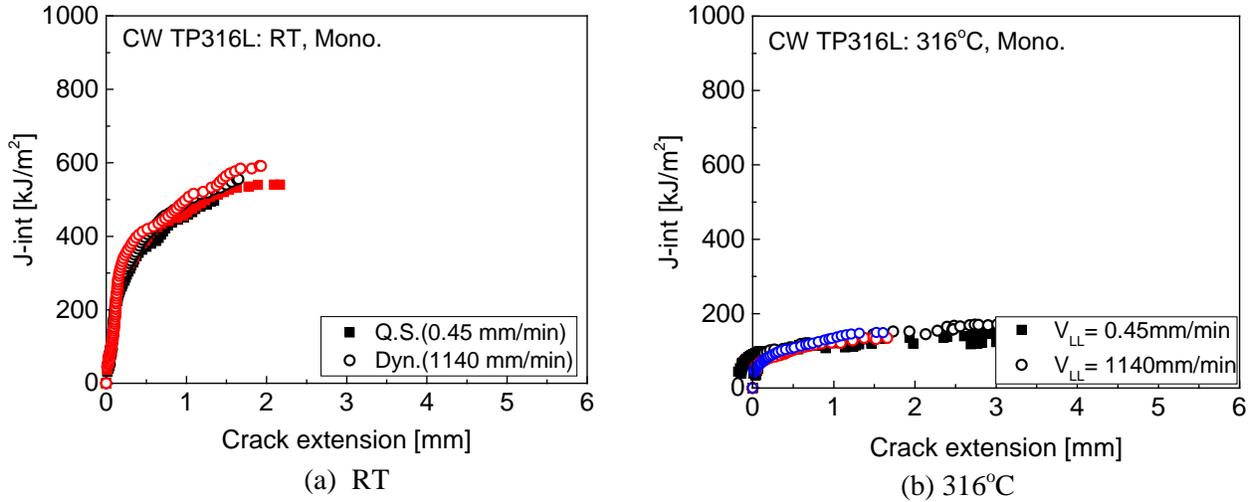
Fig. 7 Comparison of quasi-static and dynamic  $J$ - $R$  curves of cold-worked TP316L SSs
