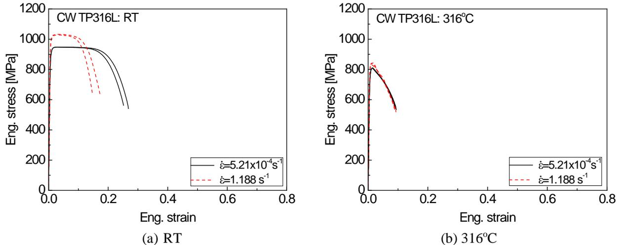
Fig. 5 Comparison of engineering stress-strain curves of cold-worked TP316L SSs at different strain rates
