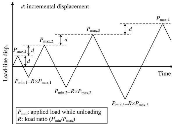
Fig. 2 Loading sequence applied to cyclic J-R fracture toughness test
