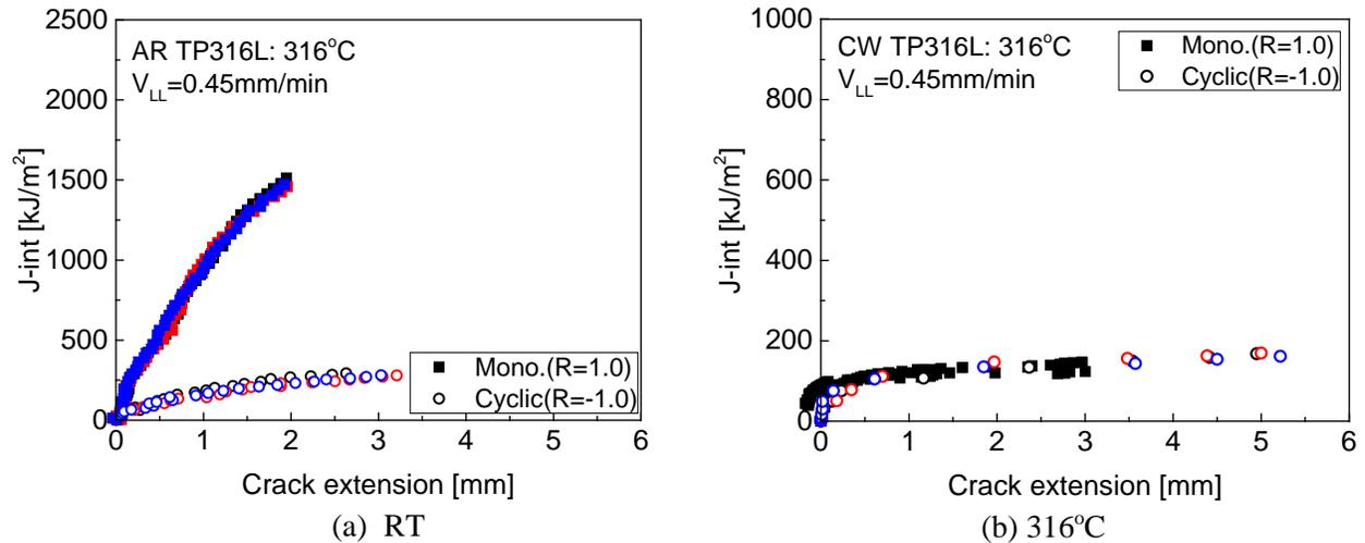
Fig. 8 Comparison of monotonic and cyclic  $J$ - $R$  curves of as-received and cold-worked TP316L SSs
