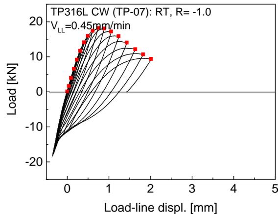
Fig. 3 A sample data obtained from cyclic J-R test
