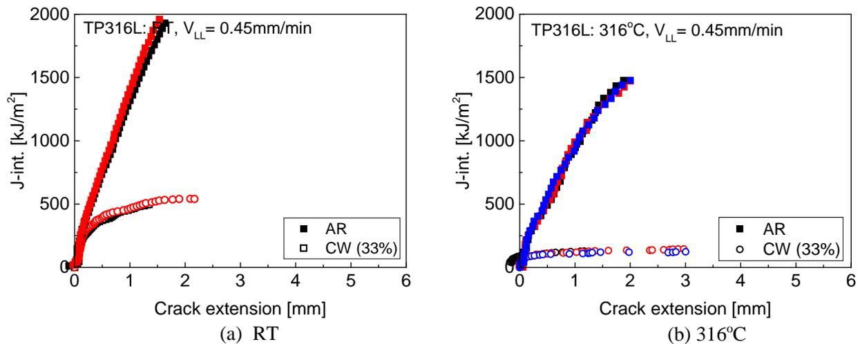
Fig. 6 Comparison of  $J$ - $R$  curves of as-received and cold-worked TP316L SSs
