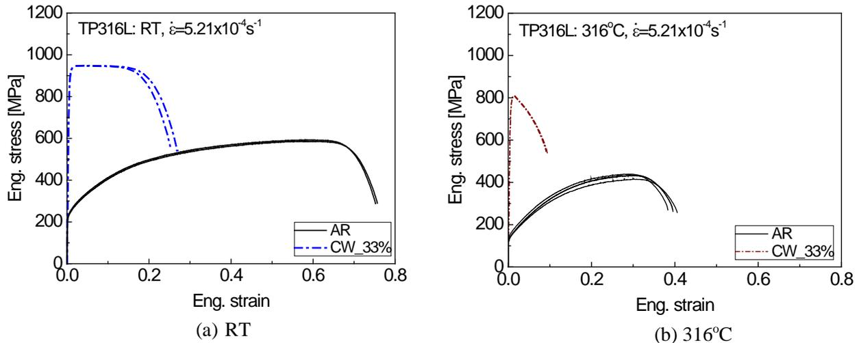
Fig. 4 Comparison of engineering stress-strain curves of as-received and cold-worked TP316L SSs
