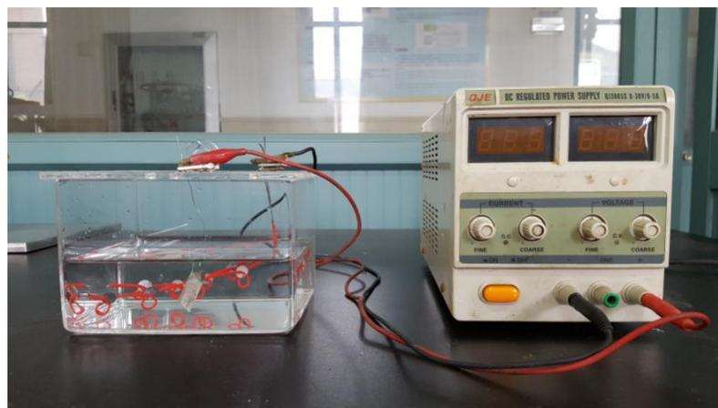
Figure 1 Electrolytic hydrogen charging test device
