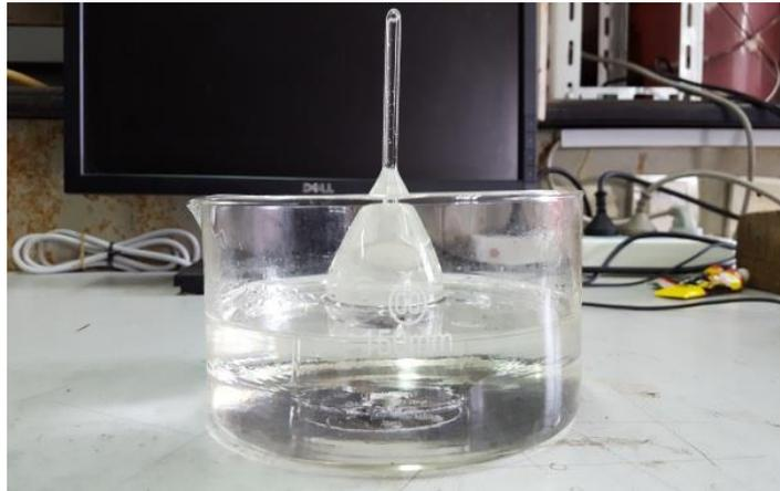
Figure 2 The device for measuring hydrogen
