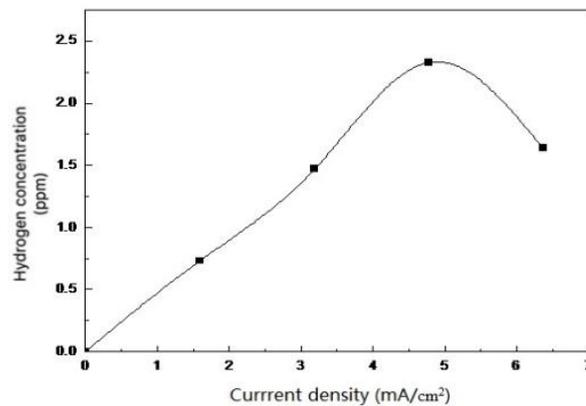
Figure 4 The relationship of hydrogen concentration and current density
