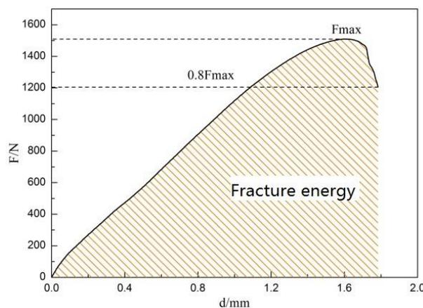
Figure 5 The schematic diagram of the fracture energy
