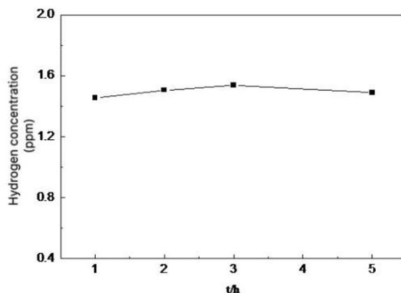
Figure 3 Relationship of charging time and hydrogen concentration
