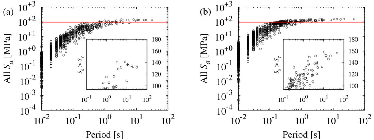
Figure 7. Results of the rainflow counting (amplitudes versus their period) for representative synthetic temperatures with fluid conditions at the D4R (a) and COR (b) points and assuming  $\Delta T = 160^\circ\text{C}$ .
