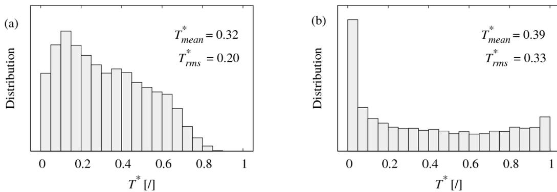
Figure 3. Histograms of the fluid temperatures at the D4R (a) and COR (b) points from the CFD-LES (Timperi, 2014).
