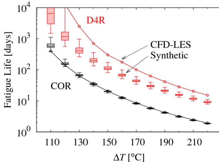
Figure 6. Results of the fatigue assessment with the CFD-LES (lines-circles) and synthetic (boxes and bars) temperatures for the fluid conditions at the D4R (red) and COR (black) points and varying  $\Delta T$ .
