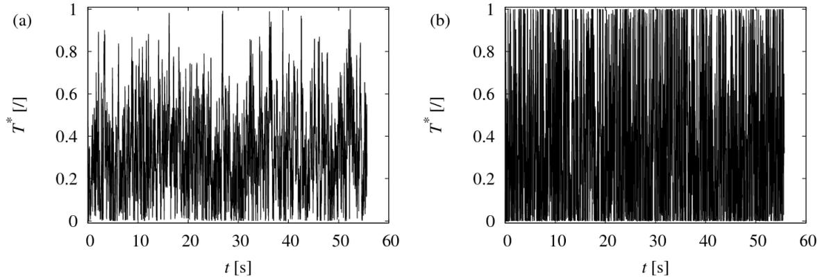
Figure 4. Representative samples of synthetic fluid temperature histories generated with the D4R (a) and COR (b) statistics.
