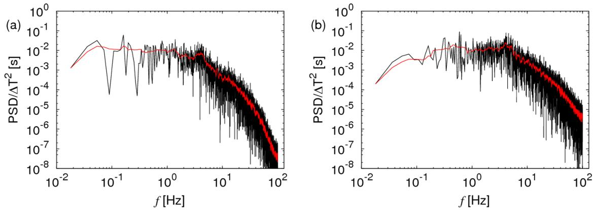
Figure 2. As computed (black) and filtered (red) PSDs of the fluid temperatures at the D4R (a) and COR (b) points from the CFD-LES (Timperi, 2014).
