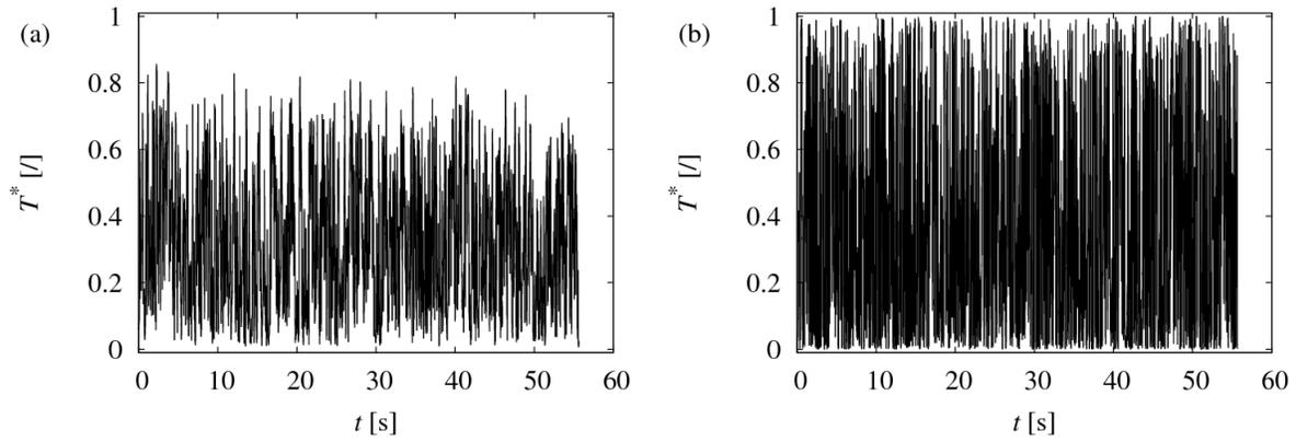
Figure 1. Fluid temperature histories at 1 mm from the pipe surface at the D4R (a) and COR (b) points from the CFD-LES (Timperi, 2014).
