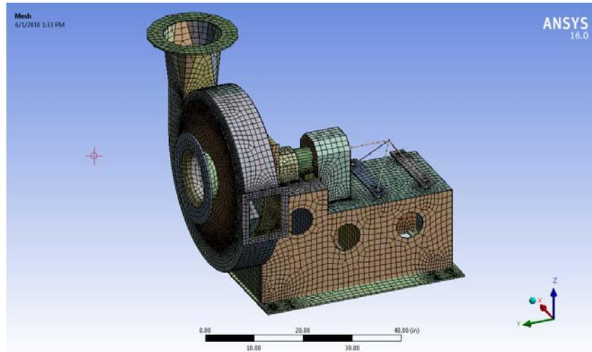
Figure 3: Isometric view of the meshed PB test fan assembly.
