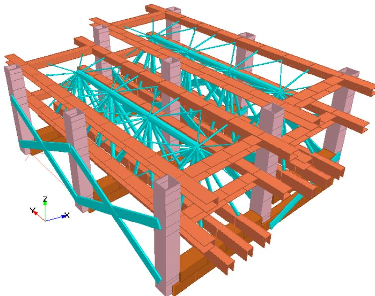
Figure 6: Isometric view of the 2-step 3-frame battery rack model.
