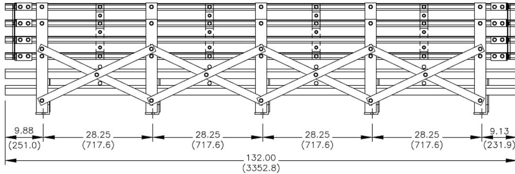
Figure 7: Side-to-side elevation view of the 2-step 5-frame battery rack.
