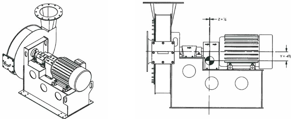
Figure 1: Isometric and elevation views of PB test fan assembly.
