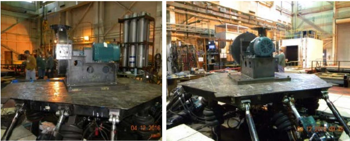
Figure 2: Final mounting of the PB test fan assembly.
