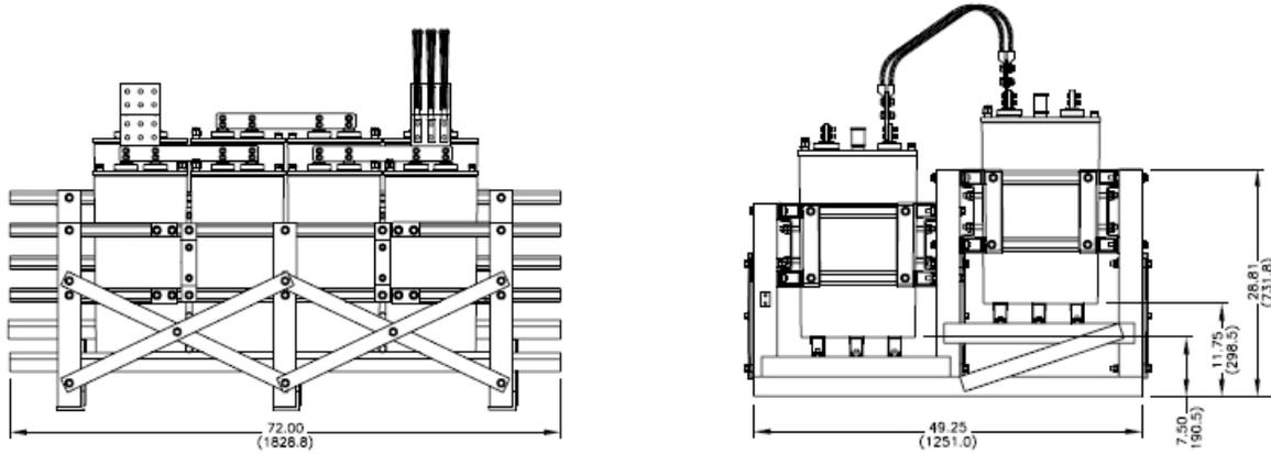
Figure 4: Elevation views of 2-step 3-frame battery rack.
