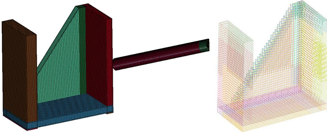
Figure 3. Finite element mesh of test V1 and its reinforcement layout
