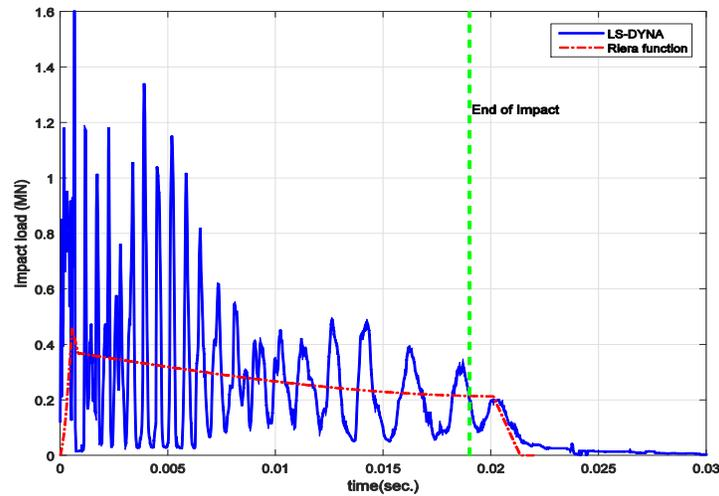
Figure 5. Comparison of impact load time histories for V1A test
