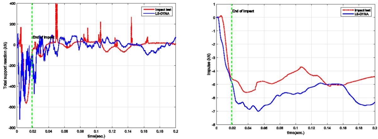
Figure 7. Comparison of horizontal support reaction forces for V1A test
