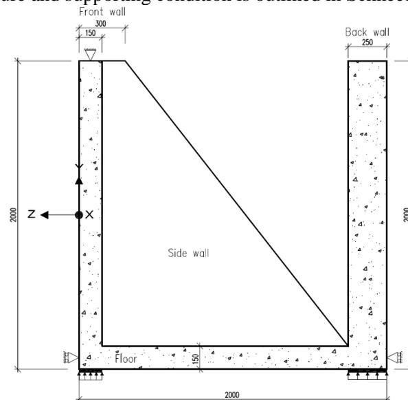
Figure 1. Experimental setup for the test series V1
