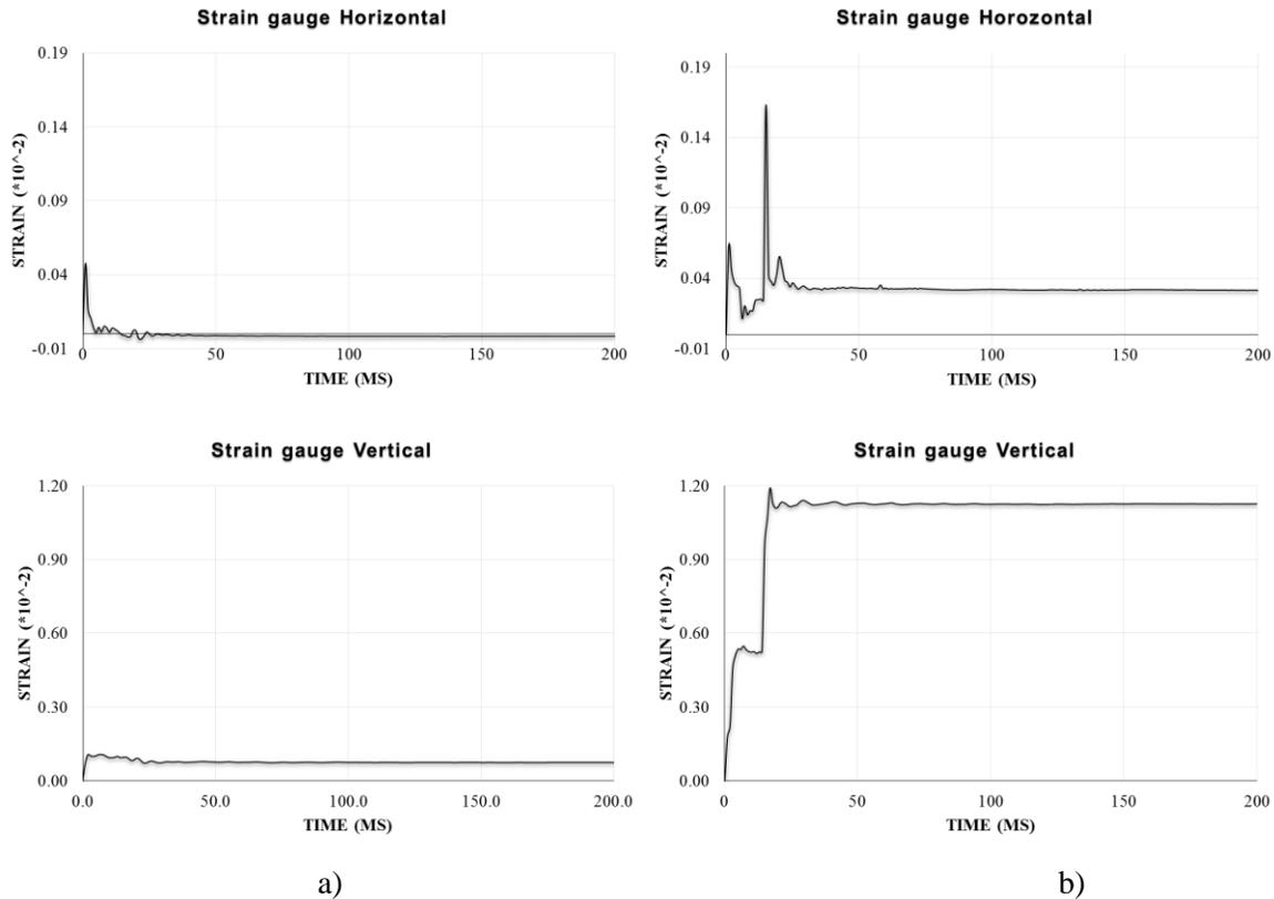
Figure 12. Predicted reinforcement strain time histories at the centre of the impacted wall for IRIS Phase 3 mock-up for a) 1st impact and b) 3rd impact
