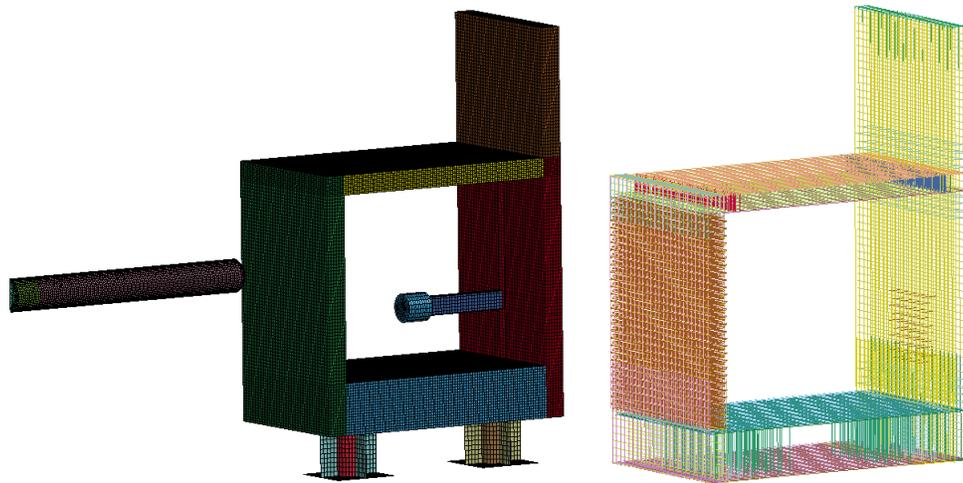
Figure 4. Finite element mesh of IRIS Phase 3 mock-up and its reinforcement layout
