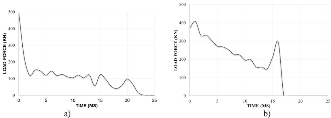
Figure 10. Predicted impact load time histories for IRIS Phase 3 mock-up for a) 1<sup>st</sup> impact and b) 3<sup>rd</sup> impact
