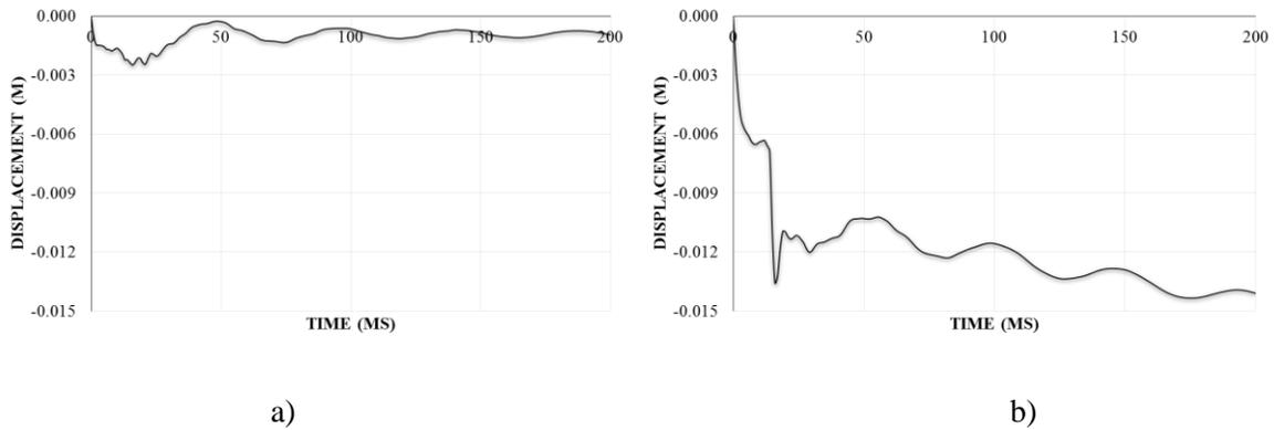
Figure 11. Predicted deflection time histories at the centre of the impacted wall for IRIS Phase 3 mock-up for a) 1st impact and b) 3rd impact
