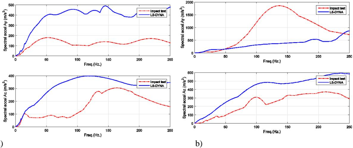
Figure 9. Acceleration spectra for V1A test at a) centre of the back wall, b) centre of the connecting floor, spectral damping 5%
