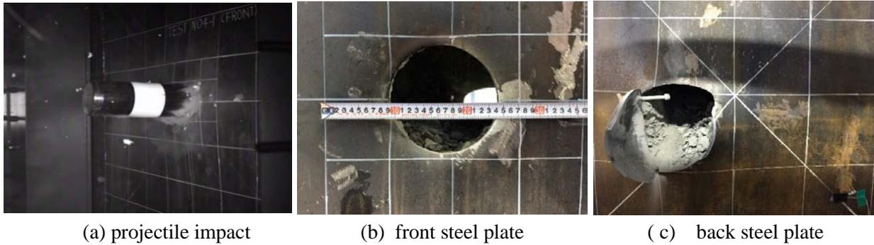
Figure 3. Test Results (SC-T360-5.0-HSA-1st)
