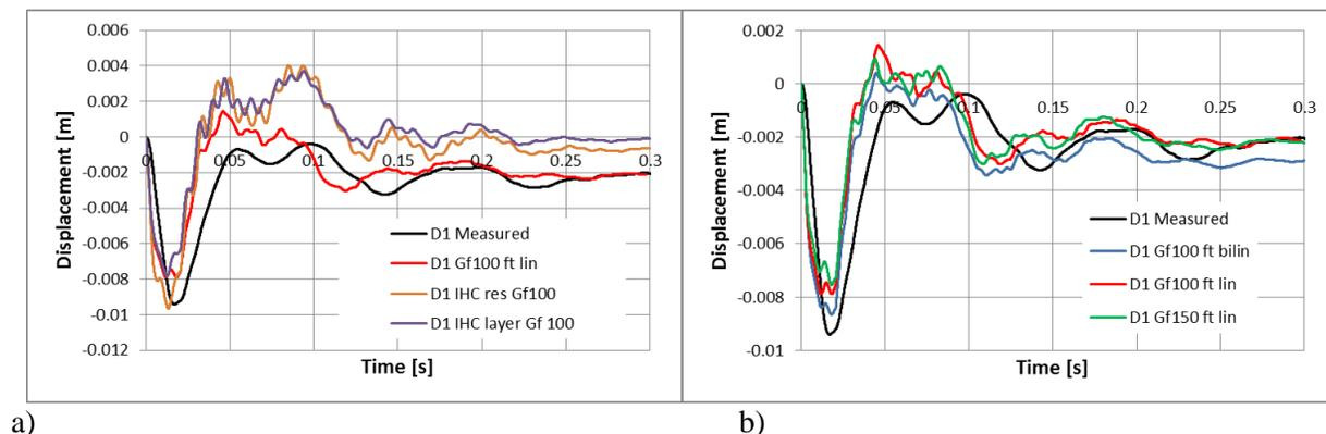
Figure 6. Horizontal displacement at the impact location, a) results obtained using different analysis codes, b) effect of tensile cracking assumption.
