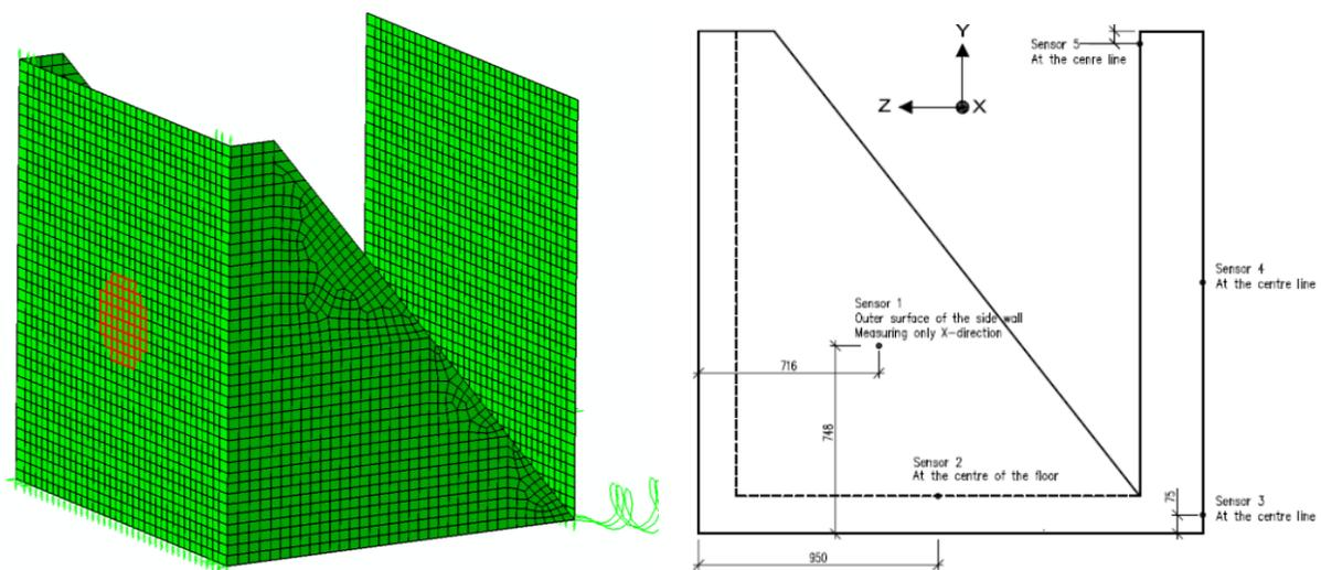
Figure 3. Shell element model and locations of accelerometers.
