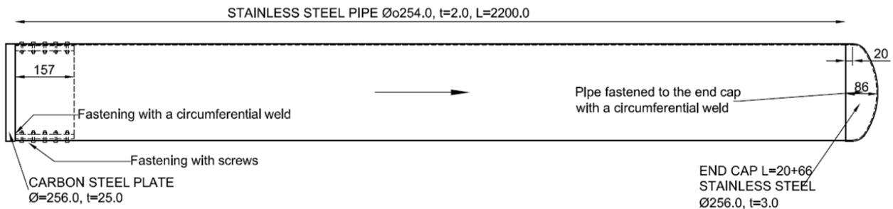
Figure 2. Stainless steel missile with a mass of 50 kg. Dimensions are in [mm].
