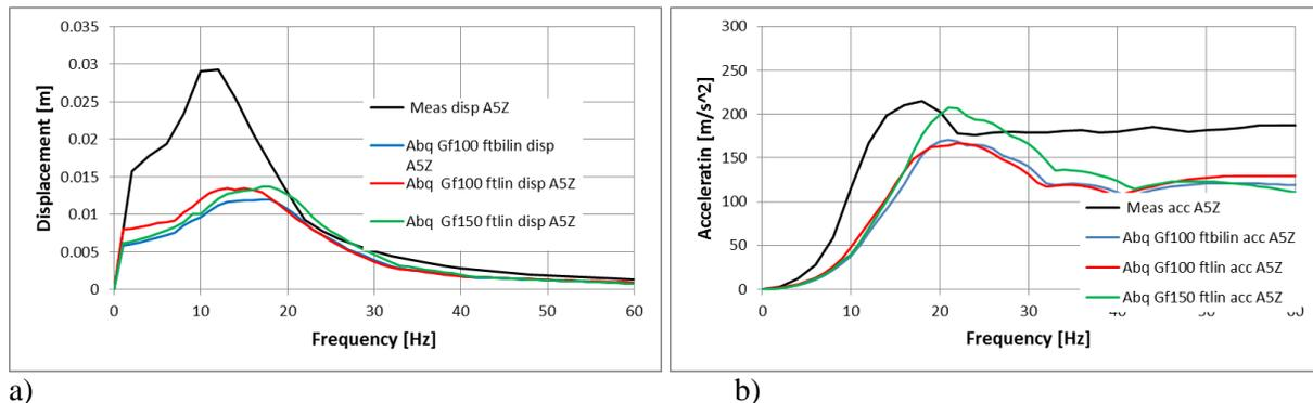
Figure 12. Displacement and acceleration spectra at the top of the rear wall in the horizontal direction showing the effect of tensile cracking assumption.
