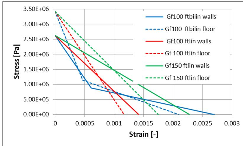
Figure 4. Tensile post-cracking properties for concrete (characteristic length 0.05 m).
