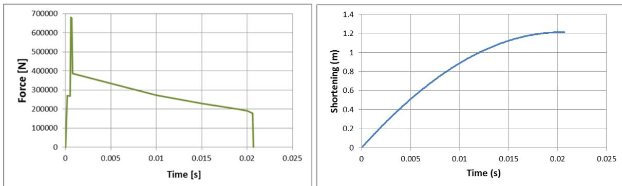
Figure 5. a) Force-time function and b) crushed length as a function of time.
