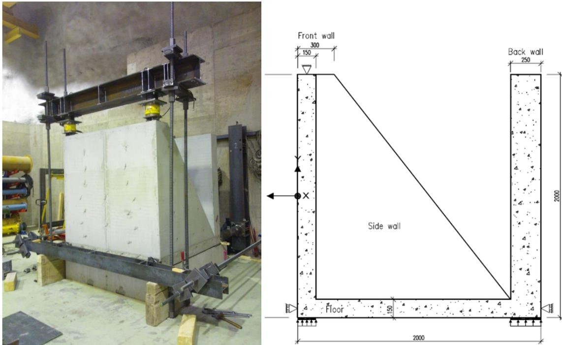
Figure 1. Reinforced concrete target with side view on the right hand side.
