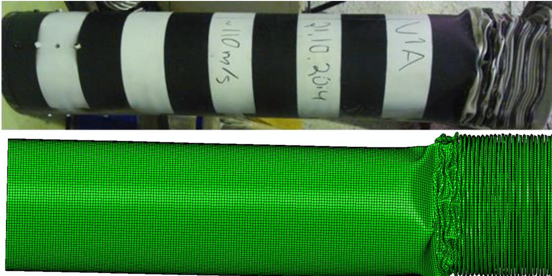
Figure 3. Deformed missile.
