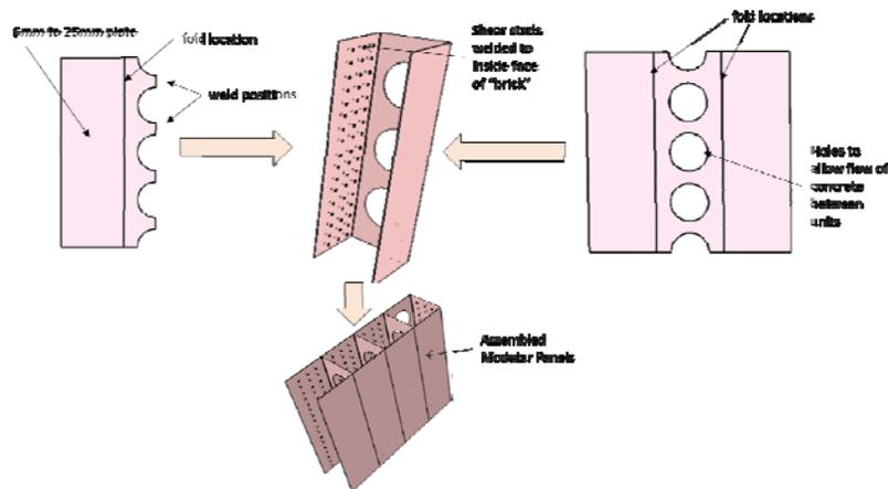
Figure 1. Fabrication and Assembly Process of Modular Panels
