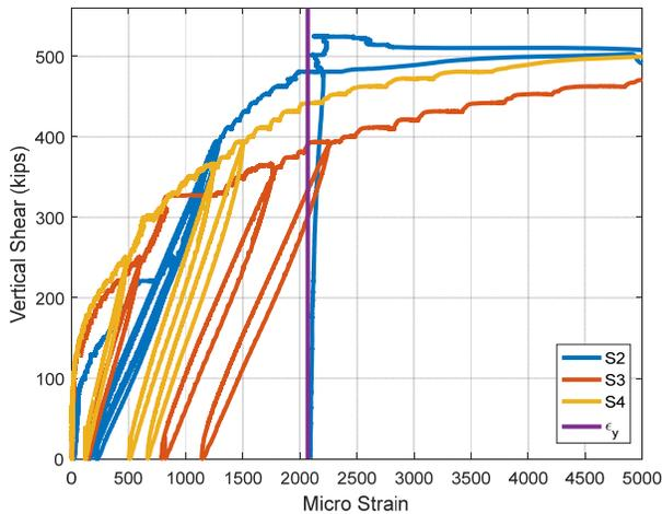
(c). North Shear Span Shear Reinforcement Strains
