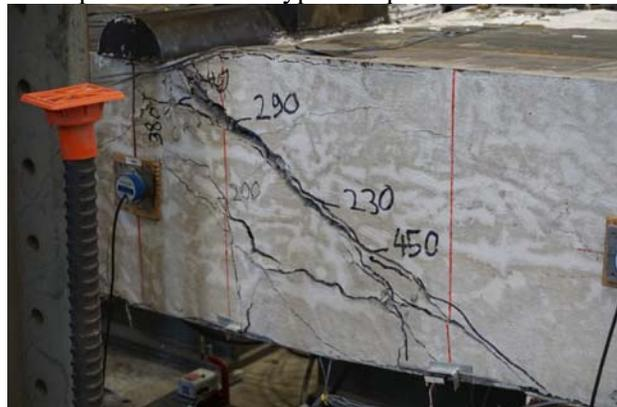
Figure 11. Shear Failure (North Shear Span – East Face) of MWS-Type 2 after Flexural Yielding
