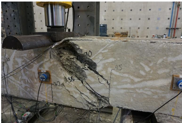
Figure 8. Shear Failure of MWS-Type 1 at 180 kips (North Shear Span – East Face)
