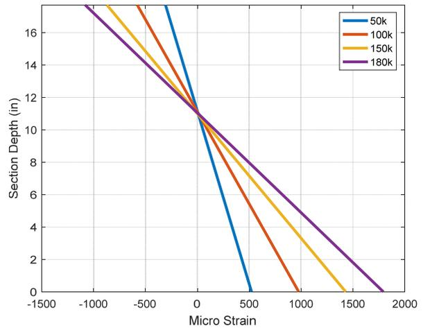
(b). Section Strains at Mid-Span (S5-S6)
