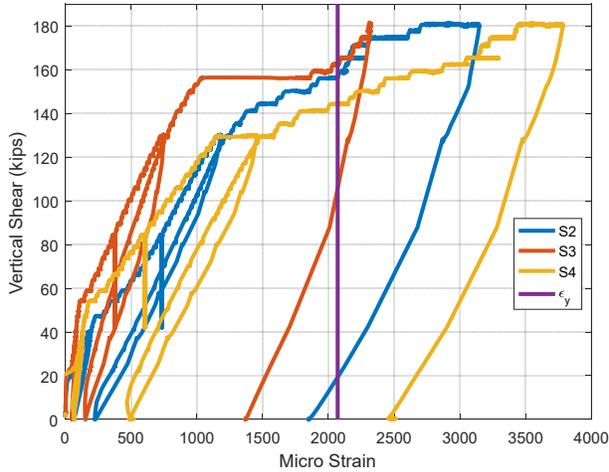
(c). North shear reinforcement strains
