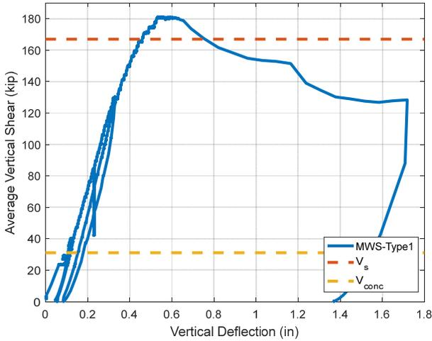
(a). Vertical Shear vs. Mid-Span Displacement
