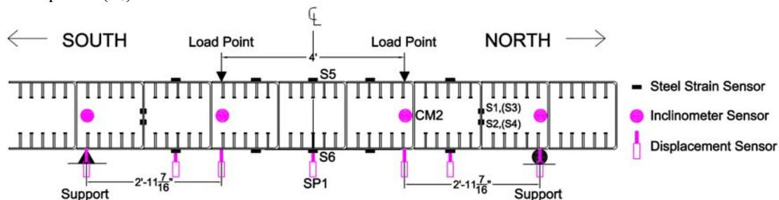
Figure 6. Specimen Drawing of MWS-Type 1
