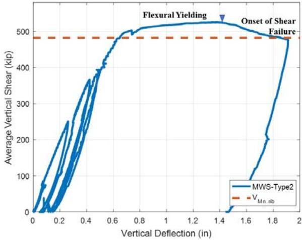
(a). Vertical Shear vs. Mid-Span Displacement
