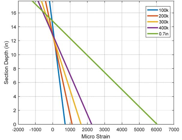
(b). Section Strains at Mid-Span (S5-S6)
