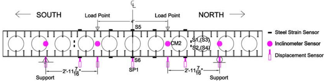
Figure 9. Specimen Drawing of MWS-Type 2
