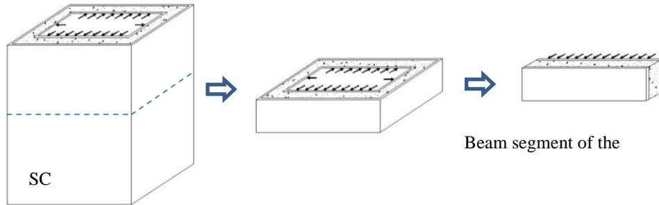
Figure 6. Schematic sketch of beam subsection taken from structural wall
