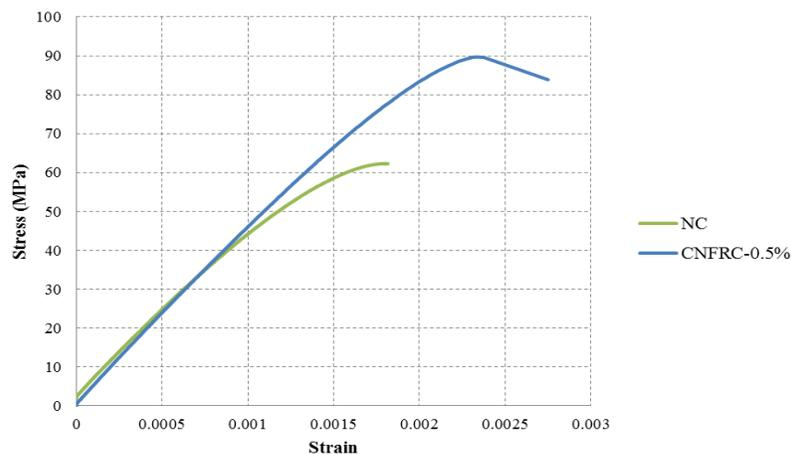
Figure 2. Cylinder Compression Test Results
