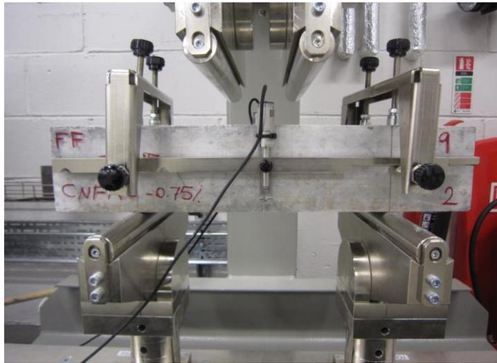
Figure 1. Flexural test set up
