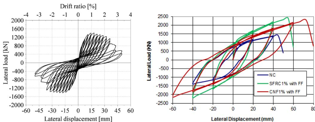
Figure 4. Load-Deflection Curve – Left: Experimental Right: Numerical. (Epackachi et al., 2004)
