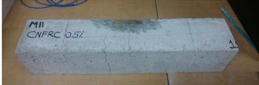
Figure 3. Failure of CNF Concrete Beam
