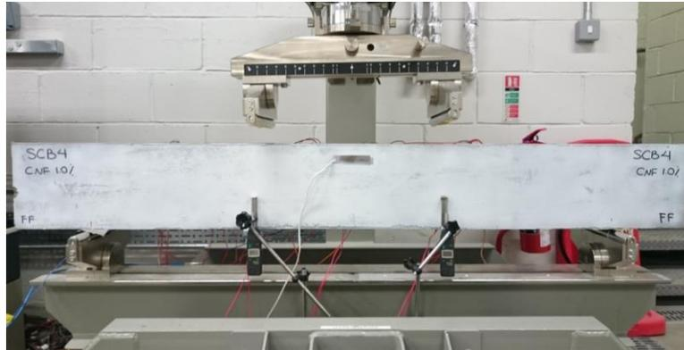
Figure 8. SC beam 4-point bending test set-up
