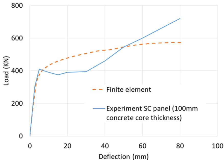
Figure 5. Load-Deflection Comparison between the Experiment Results and the Fibre Beam Element where 1% Steel Fibre is Considered (Sohel and Liew, 2014)
