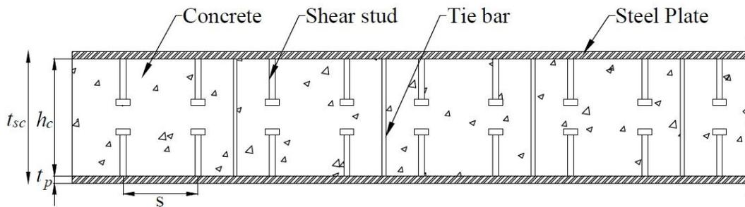
Figure 7. Schematic illustration of SC wall section
