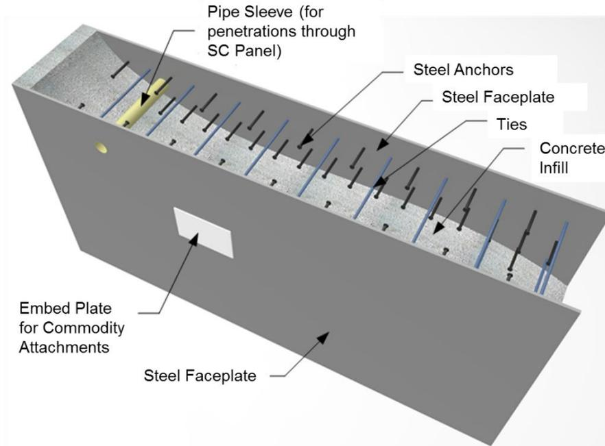
Figure 1. Basic SC Wall without Linear Reinforcing Elements (from AISC, 2015)
