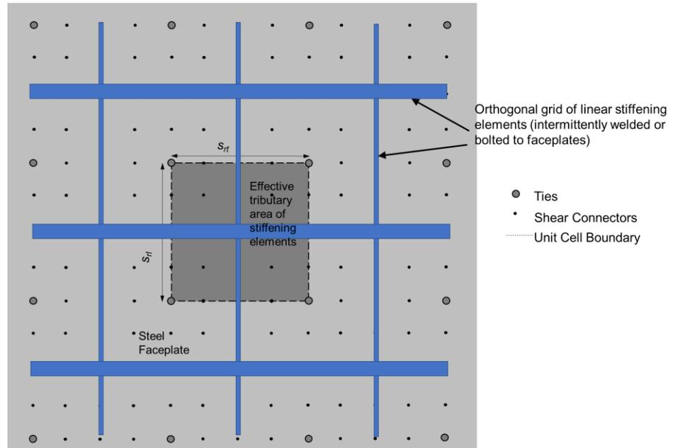
Figure 2. Elevation view of a typical SC wall with linear reinforcing elements (faceplate not shown for clarity)
