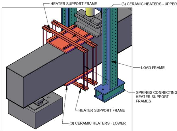
Figure 3 – Accident Thermal Test Setup
