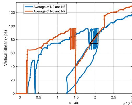
Figure 10 – Average shear force vs. average shear strain
