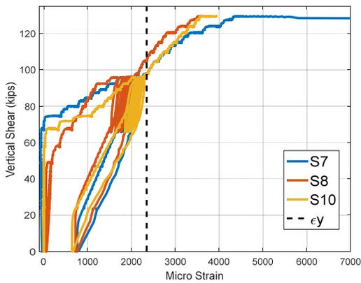
Figure 9 – Average shear force vs. shear reinforcement strains
