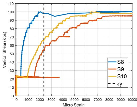
Figure 17 – Average shear force vs. shear reinforcement strains
