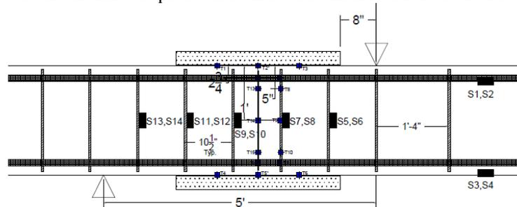
Figure 6 - Locations of Strain gauges and Thermocouples in the Heated Region
