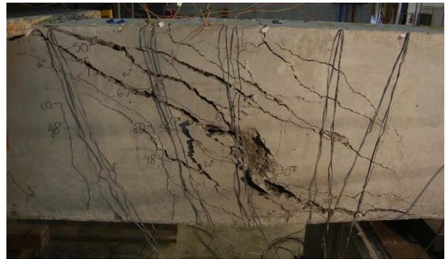
Figure 8 - Diagonal Shear Failure in the Shear Span (East Face)
