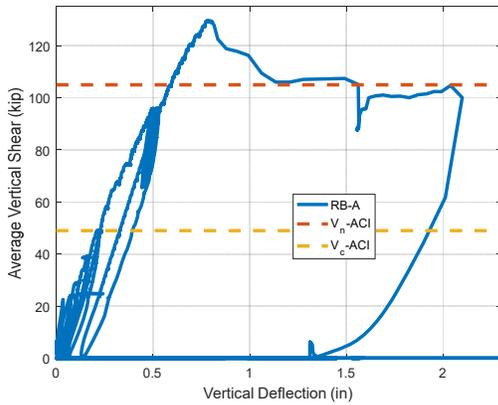
Figure 7 – Average shear force vs. mid-span displacement
