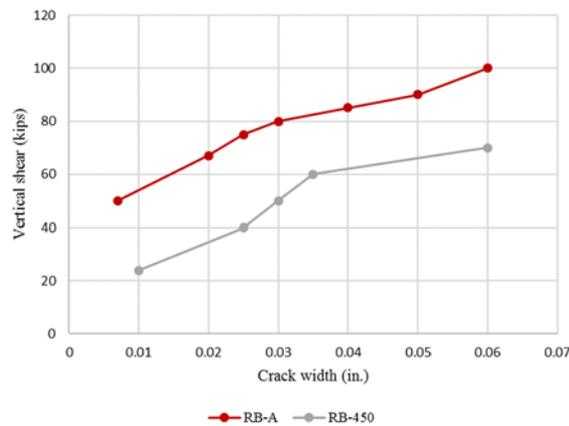
Figure 20 – Comparison between Shear Crack Widths at different loads
