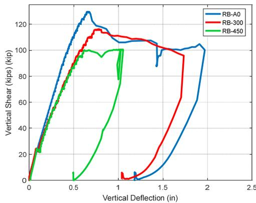
Figure 15 – Average load vs. mid-span displacement
