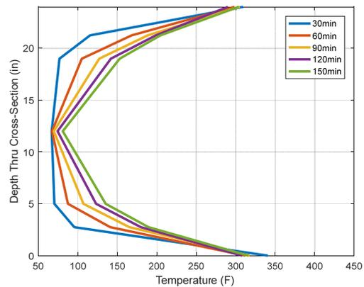
Figure 12 – Through-depth temperature distribution
