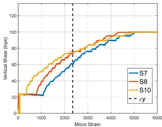
Figure 13 – Average shear force vs. shear reinforcement strains
