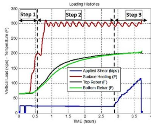
Figure 4 –Loading History and Rebar Temperatures of RB-300
