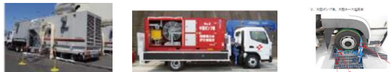
Figure3. Mobile SA equipment (Left: Power car, Center: Fire truck), Right: Status of lashing of SA equipment
