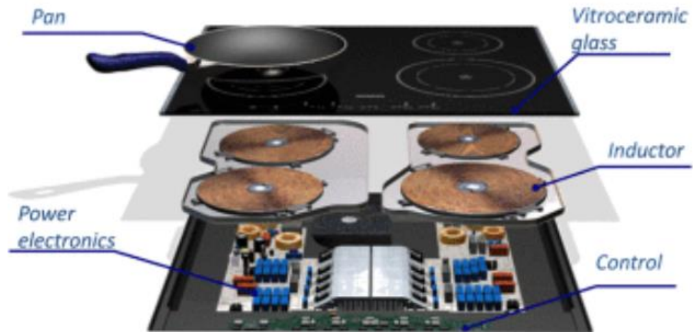
Figure 2.7. Exploded view of induction heating appliances (Lucia, O., Acero, J., Carretero, C., & Burdio, J. M., 2013)
