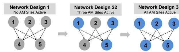
Figure 3: Example layout of 3 different NDs with different combinations of AM Locations at DCs and SLs (AM site indicated by a blue circle)
