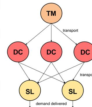
Figure 2: A visual representation of the network with flow of products moving from TM to DCs and exiting the system through the SLs
