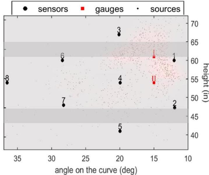
Figure 3. Localization of AE sources
