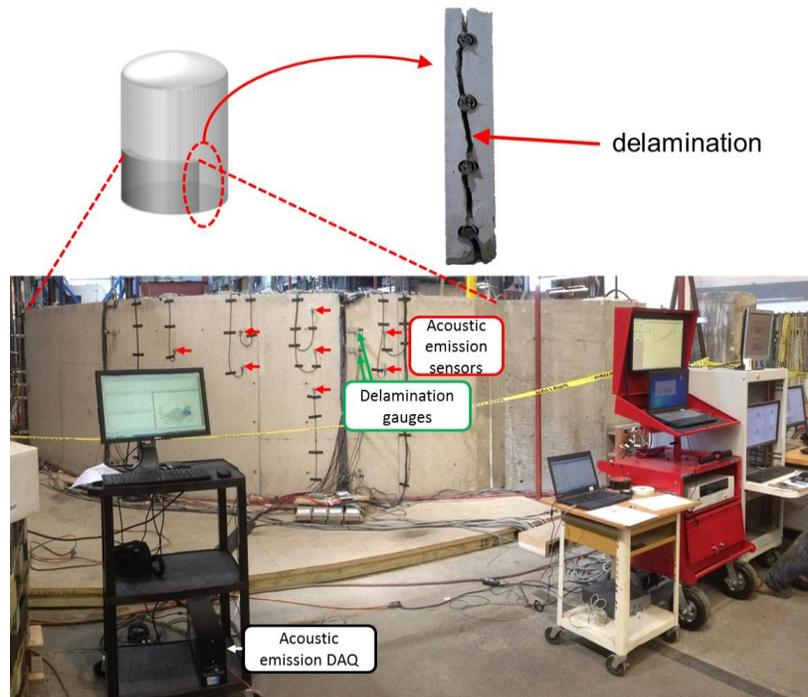
Figure 2. Experimental setup
