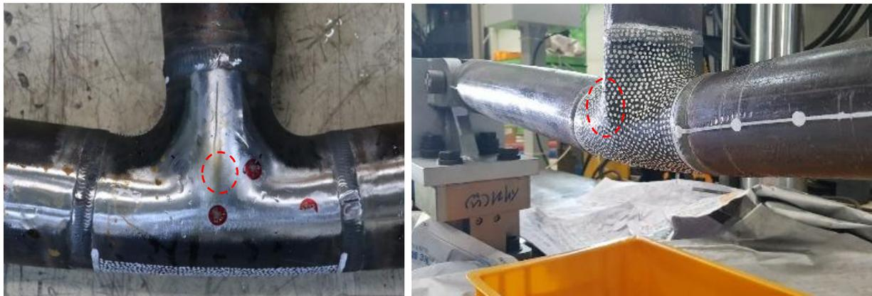
Figure 3. Leakage point of carbon steel pipe tee under in-plane cyclic loading
