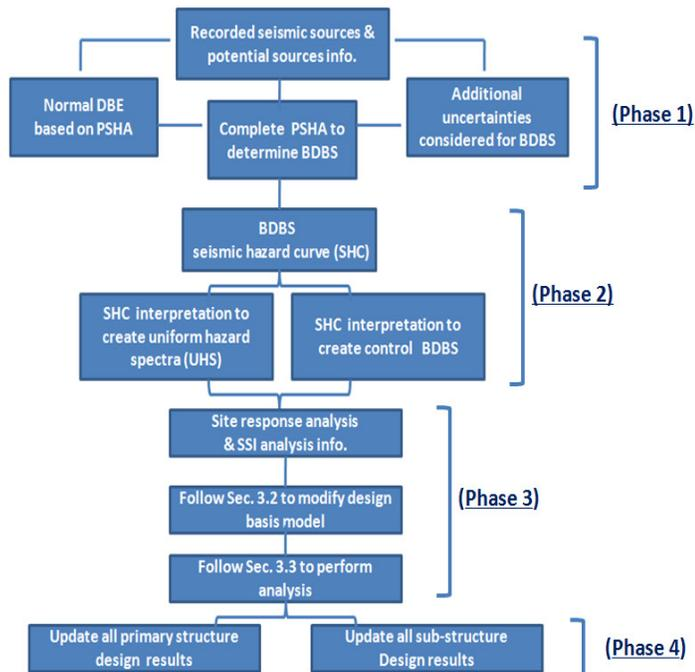
Figure 7: Integrated complete probabilistic framework for BDBS design
