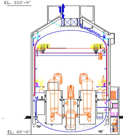
Figure 3: Complex structure – system – component within NI
