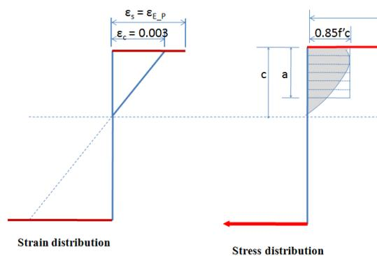
Figure 10: SC wall concrete strain-stress relationships
