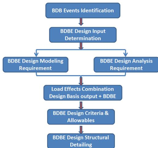
Figure 5: The basic design flowchart of BDBE for new NPPs
