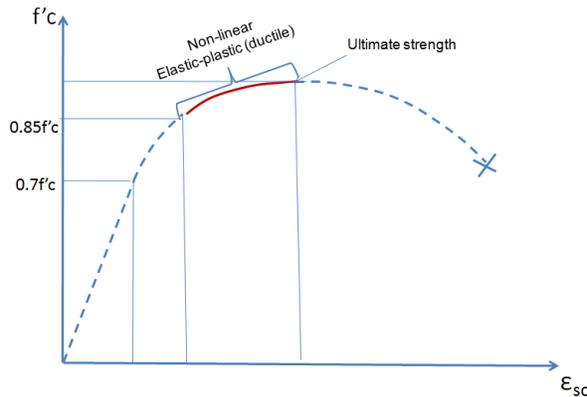
Figure 8: SC wall concrete strain-stress relationships
