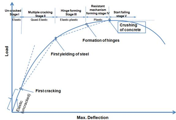
Figure 9: SC wall concrete strain-stress relationships
