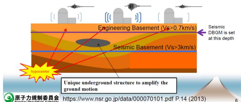
Figure 4: Design Basis Ground Motion (DBGM)
