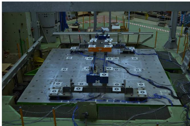
Figure 4: The crane bridge on the AZALÉE shaking table - CEA/Saclay
