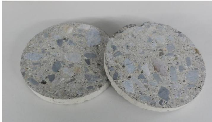
Fig. 1 Photograph of the sliced concrete samples.
