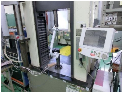
Figure 4. Setup of the static loading test
