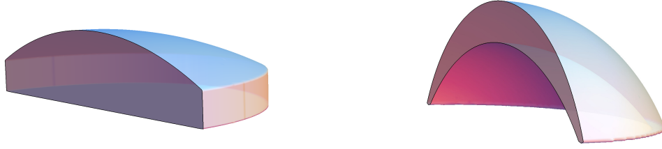
Figure 6.1: Renderings of the aspheric lens (left) and the toric lens (right) from the design equations in Section 2.3.
