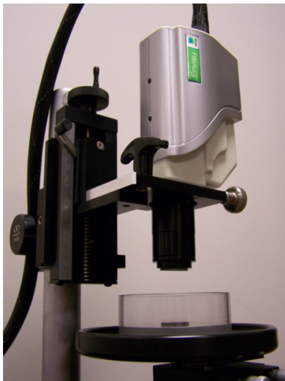
Figure 2.3: Envisu metrology assembly with handheld R4410 OCT probe [51].
