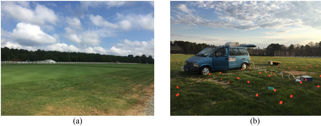
Figure 2.1: (a) The view from one of the fields at Lake Wheeler Turfgrass Field Laboratory; (b) Mobile laboratory (modified Ford Aerostar minivan) was parked in the middle of the sampling field. The mobile laboratory was about 100 ft away from the office, from where the electricity to power the instruments and air conditioner was supplied.
