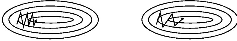
Figure 2.6: Graphics showing the convergence of gradient descent without momentum (left) and with momentum (right) [50].
