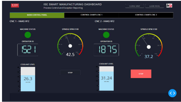
Fig. 4. Dashboard of key metrics transferred from two CNC machines in real-time
