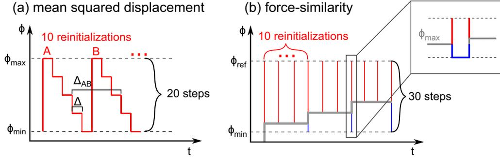
FIG. 2. (a) Schematic representation of the protocol used to determine the cage size  $\Delta$  and the mean cage separation  $\Delta_{AB}$  via the MSD. (b) Schematic representation of the protocol used to determine the persistence of interparticle contacts via the force-similarity analysis.
