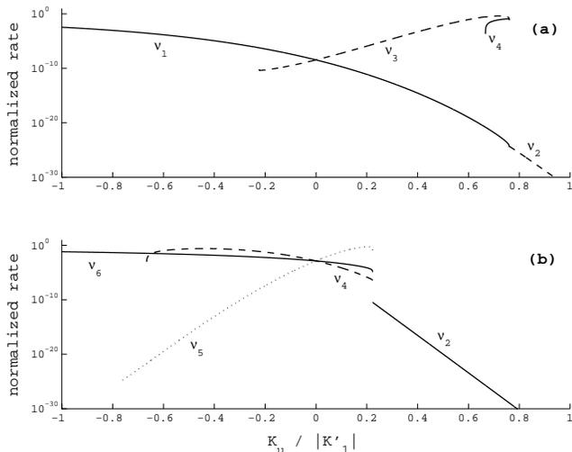
FIG. 5: Single-barrier relaxation rates  $\nu_i$  for (a) Fe ( $M_s = 1.72 \times 10^6$  kA/m,  $K'_1 = 4.8 \times 10^4$  Jm<sup>-3</sup>) and (b) Ni ( $M_s = 4.85 \times 10^5$  kA/m,  $K'_1 = -5 \times 10^3$  Jm<sup>-3</sup>). In both plots,  $|K'_1|v/kT = 80$ ,  $\alpha = 0.1$  and the rates are normalized by  $2\pi M_s / |\gamma_0 K'_1|$ .
