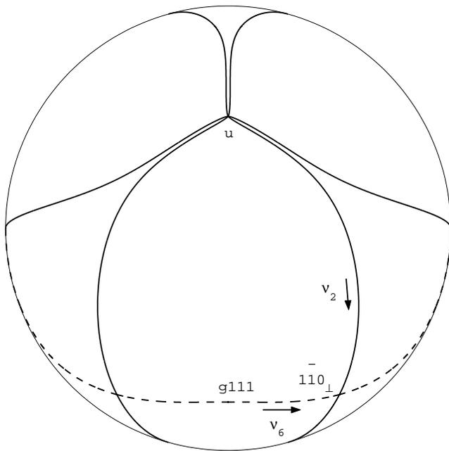
FIG. 9: Equilibrium states and their connections for  $\kappa = 1$  and easy axis in the  $[111]$  direction. The conventions are the same as for Fig. 6.
