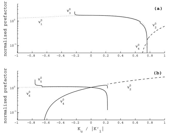
FIG. 4: Prefactors for the single-barrier relaxation rates  $\nu_i$  listed in Table I. The prefactors are normalized by  $2\pi M_s / |\gamma'_0 K'_1|$  and the parameters  $\alpha = 0.1$ ,  $|K'_1|v/kT = 80$  are used. (a)  $K'_1 > 0$ . (b)  $K'_1 < 0$ .
