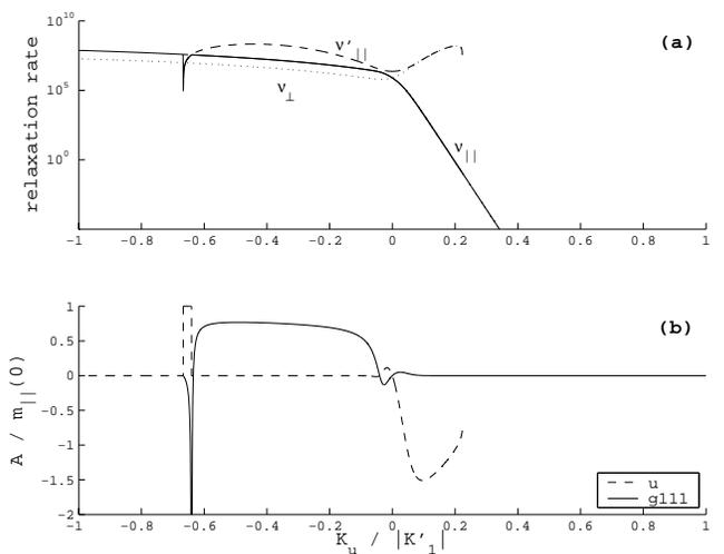
FIG. 12: (a) Relaxation rates for nickel (same parameters as in Fig. 5b). (b) Parameter  $A$  in the prefactor for rates  $\nu_{\parallel}$ ,  $\nu'_{\parallel}$ . As depicted, some rates are only defined for a particular starting state.
