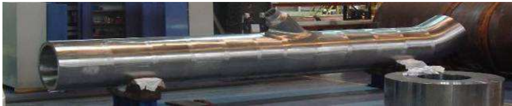
Fig. 3: Cold Leg forged from a solid ingot
