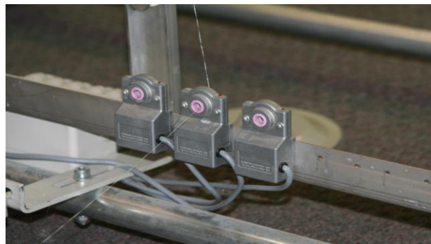
Figure 3.3: Ceramic guide with an electronic yarn breakage detector
