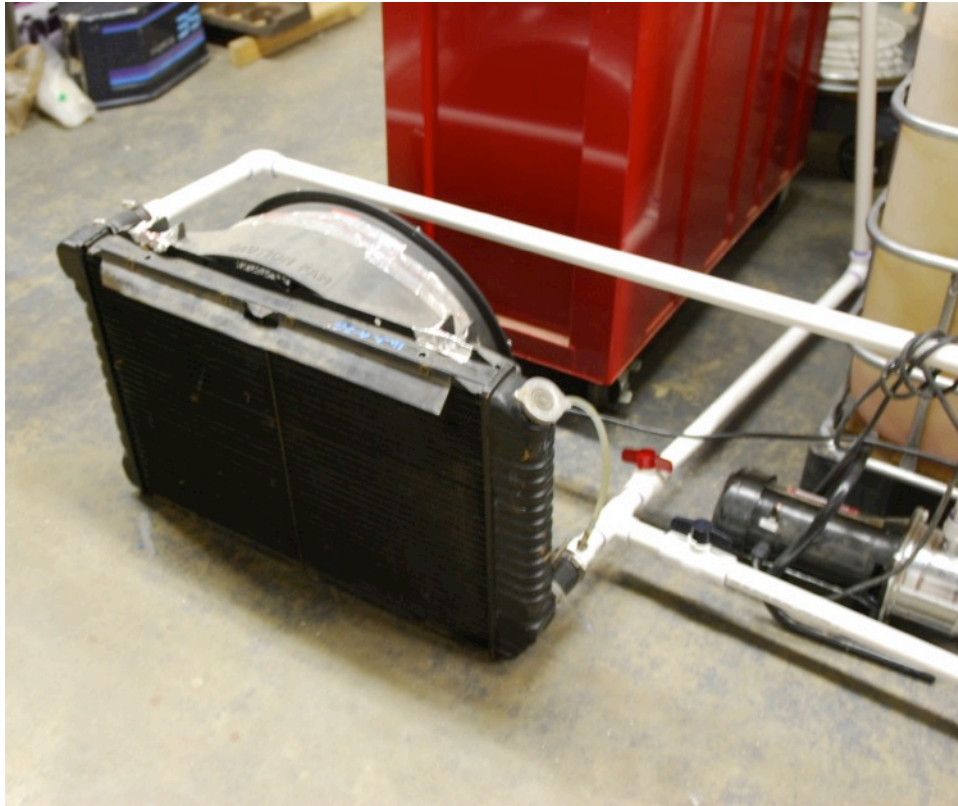
Figure 7 - Fan and radiator system with reservoir cooling pump
