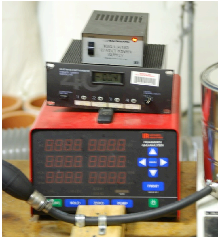
Figure 24 - Mass flow meter power supply with digital display and exhaust gas analyzer
