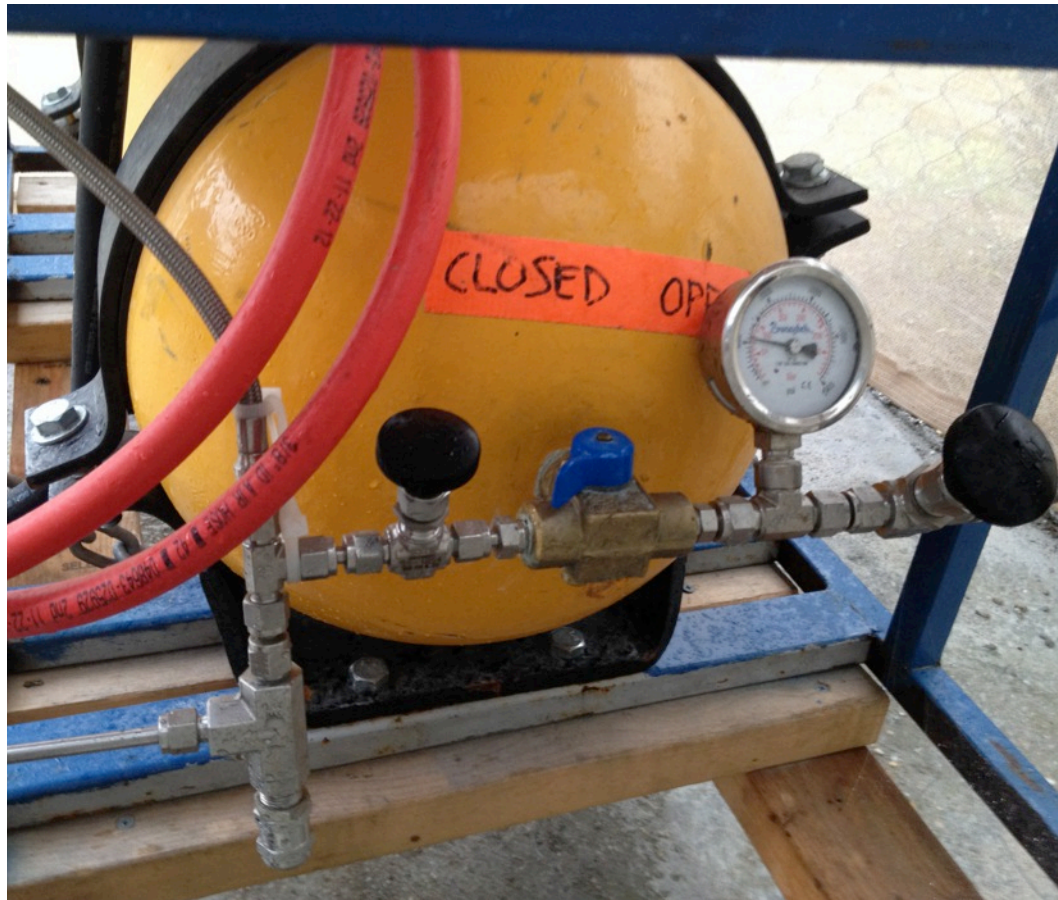
Figure 17 - CNG tank refueling and delivery high-pressure valve and tubing configuration
