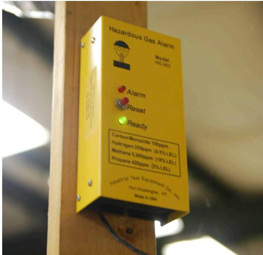
Figure 13 - Hazardous gas alarm
