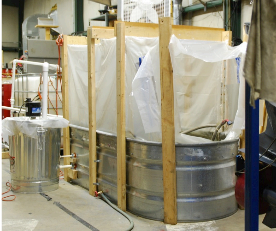
Figure 8 - Engine-cooling tank and exhaust shroud
