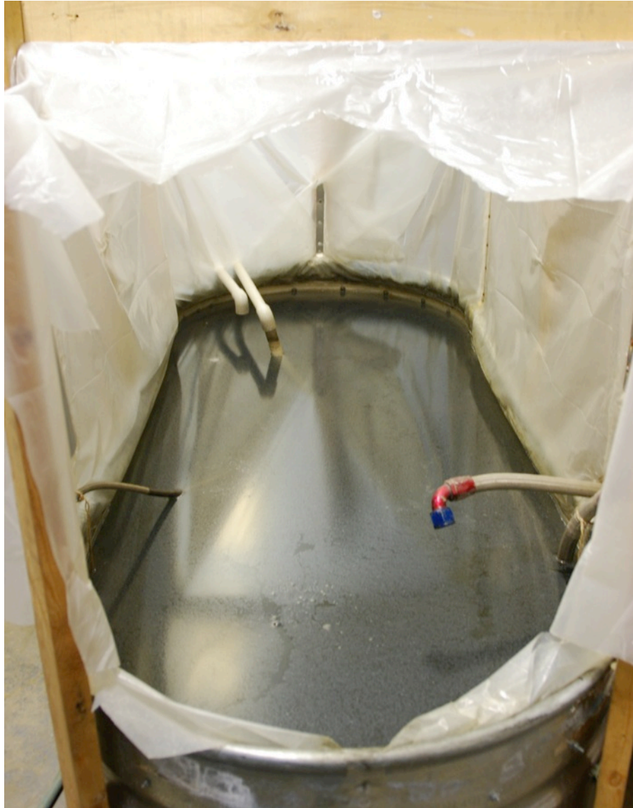
Figure 12 - Engine cooling-tank insertion point with dynamometer absorber hook-ups
