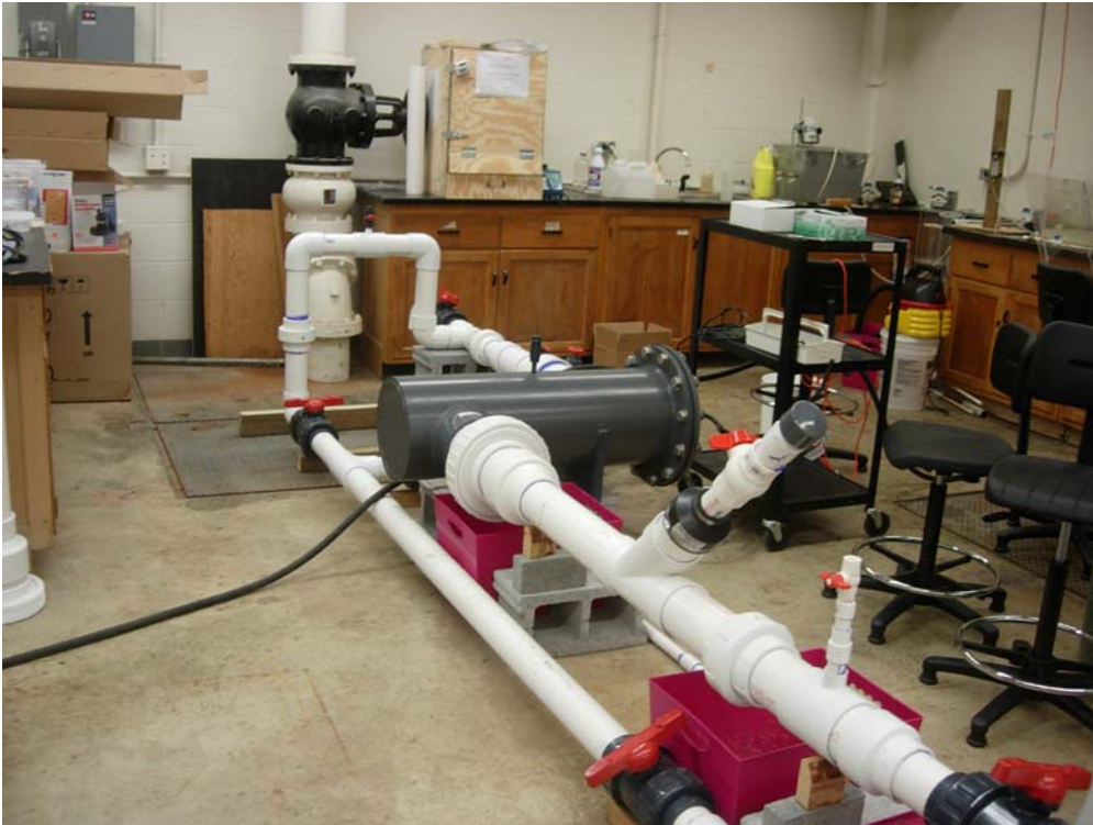
Figure 3: Photograph of pilot test that displaying injecting and excluding Lagrangian UV sensor
