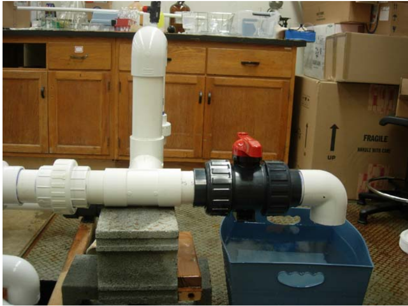
Figure 5: Outlet part that Lagrangian UV sensor get out of the UV system
