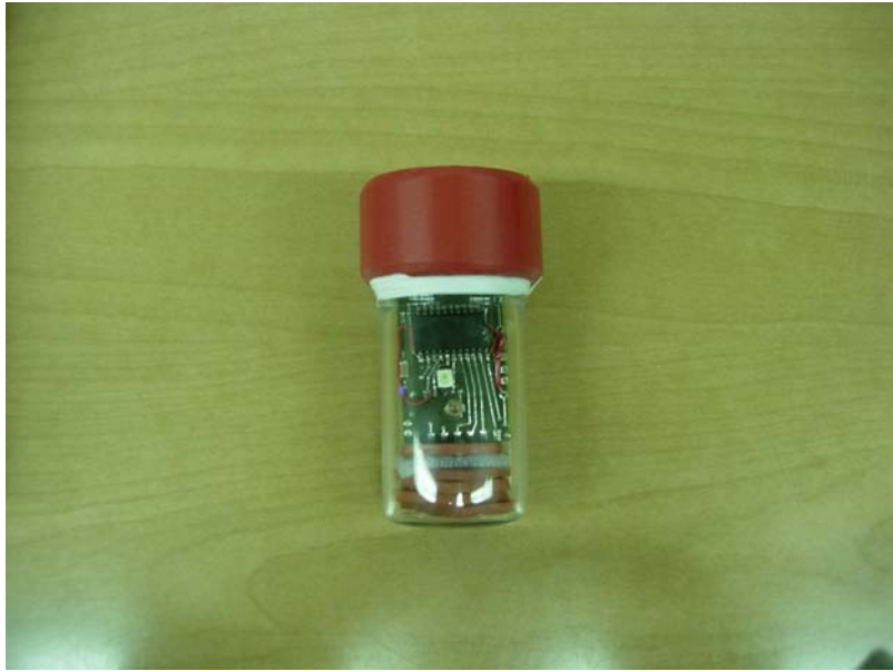
Figure 6: Quartz tube as a Body of Lagrangian UV sensor
