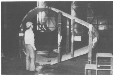
Photo 1. Shaped sectorial rigid ring of the vacuum vessel.
