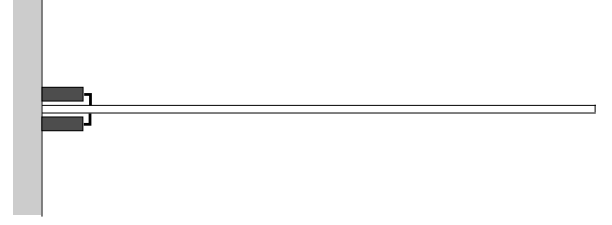
Figure 4. Cantilever beam with magnetostrictive actuators.
