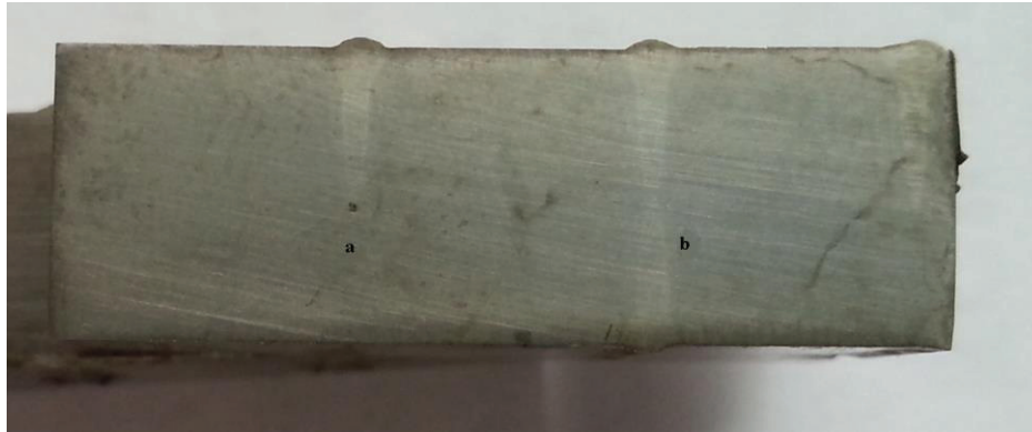
a – unilateral welding; b – two-side welding.
