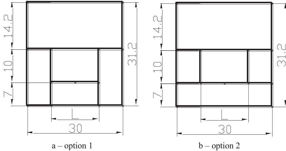
Figure 2. The layout chart for casing elements and inserts in reconstituted CT specimens with L \times 10 \times 10 mm insert size: (a) – L=10 mm, (b) – L=20 mm.
