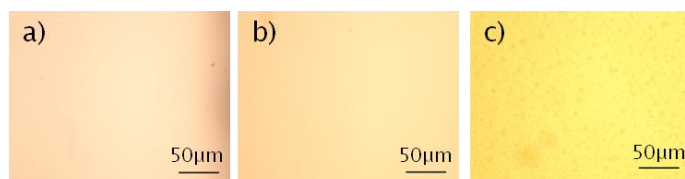
Figure 2.2. Optical micrographs of (a) Neat PAN in DMSO, (b) sonicated lignin in DMSO, and (c) lignin/PAN in DMSO.
