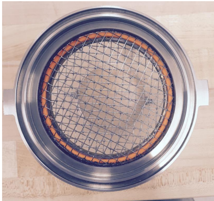
Figure 4.7: Bottom View of a Ring inside the Compression Tube
