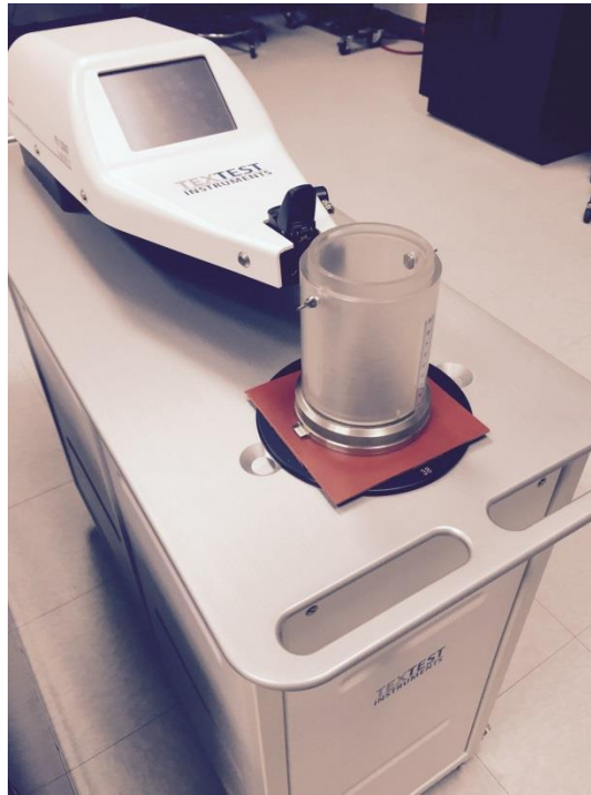
Figure 4.5: The Compression Tube Being Used with the FX-3300 Tester & Rubber Sheeting
