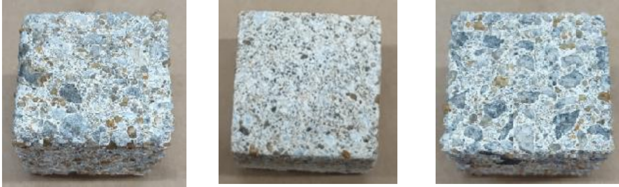
Figure 4.11 Visual inspection of LST4 (left), LSI5.0 (center), and GST4 (right) after 30 days of testing
