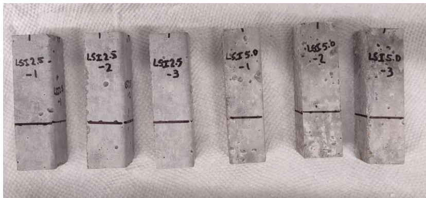
Figure 4.17 Concrete samples before the start of the FOG deposit formation test
