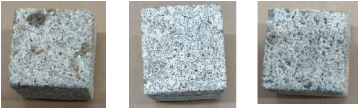
Figure 4.9 Visual inspection of LST4 (left), LSI5.0 (center), and GST4 (right) after 14 days of testing
