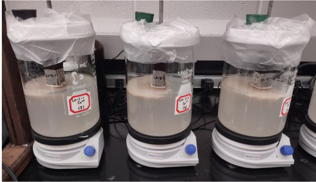
Figure 4.13 FOG deposit formation test of control concrete with limestone aggregates at 3 days
