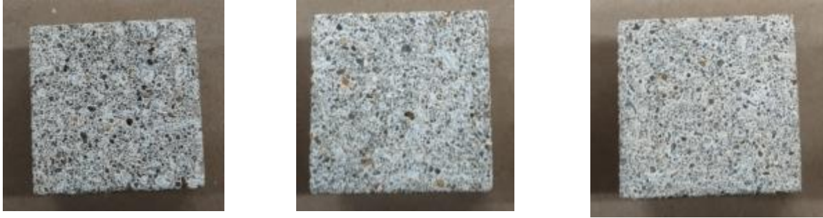
Figure 4.8 Visual inspection of LO (left), LSI2.5 (center), and GO (right) after 14 days of testing
