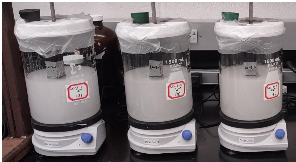
Figure 4.12 FOG deposit formation test of control concrete with limestone aggregates at 0 days
