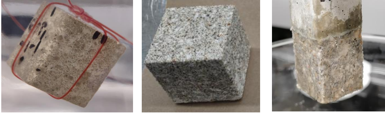
Figure 4.19 Concrete samples; after 50 days of leaching test (left), after 14 days of acid attack (center), after 20 days of FOG deposit formation test (right)
