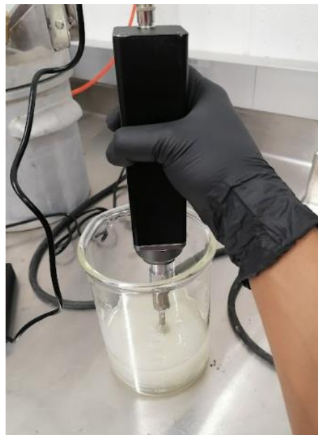
Figure 3.1 Homogenization of SME and water with an ultrasonic probe
