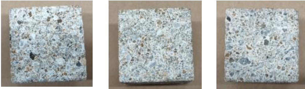
Figure 4.10 Visual inspection of LO (left), LSI2.5 (center), and GO (right) after 30 days of testing
