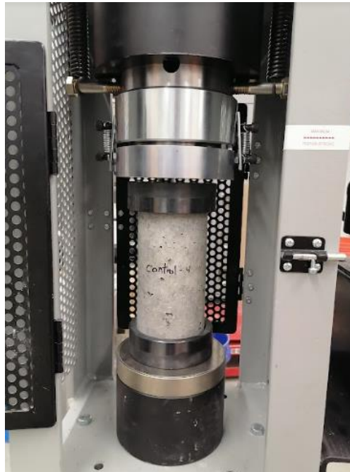
Figure 3.4 Compression test on cylindrical samples
