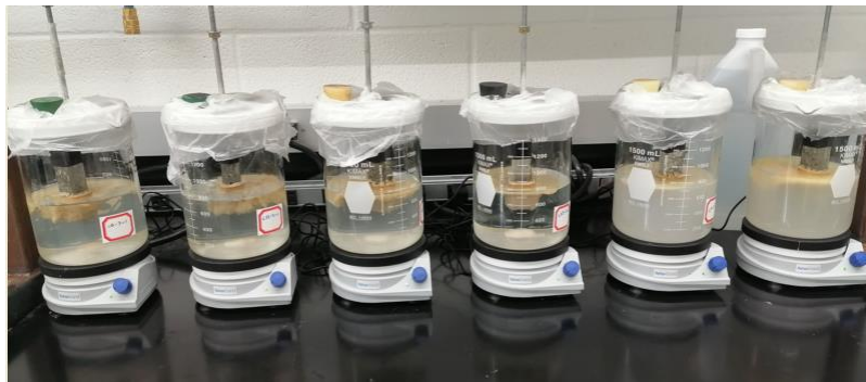
Figure 3.9 Experimental setup for the FOG deposit formation test
