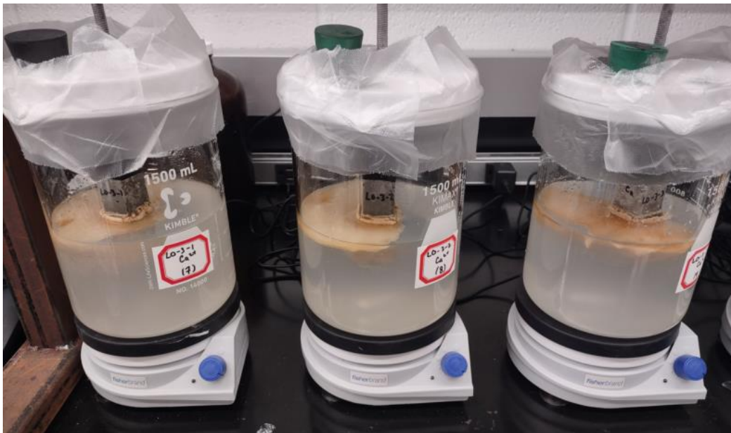
Figure 4.16 FOG deposit formation test of control concrete with limestone aggregates at 20 days
