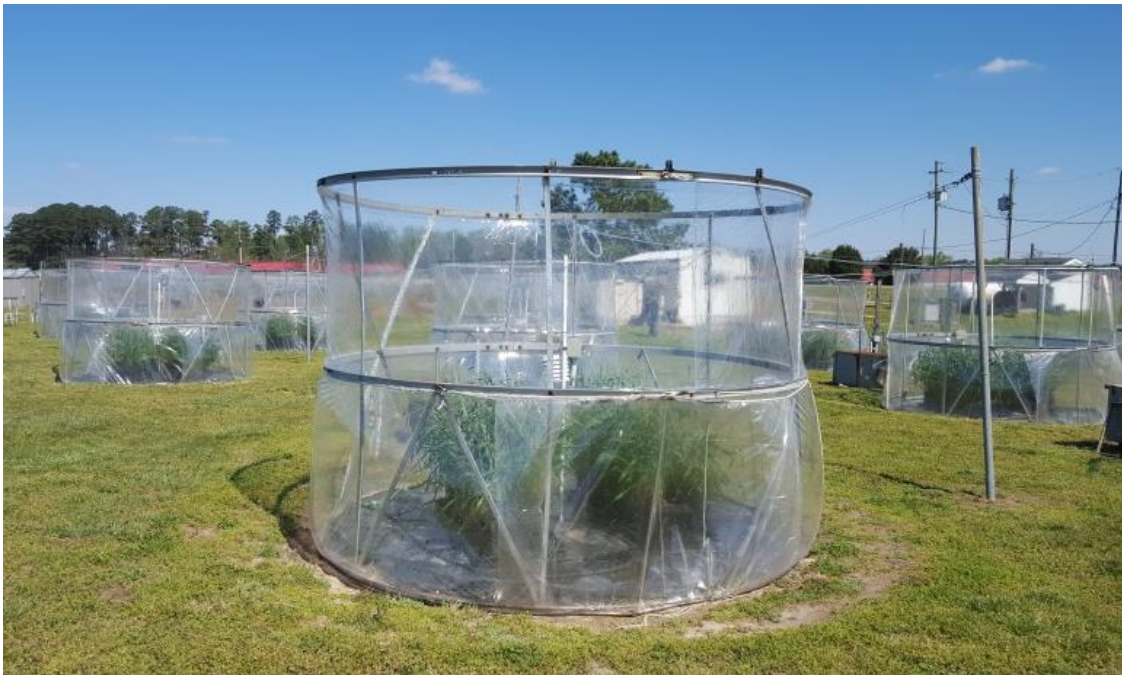
Figure (4): Open-top Chambers (OTCs). Plant Science Unite Field, USDA-ARS, Raleigh, NC, U.S.A.
